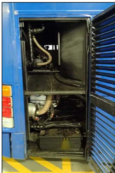
Figure 11. Photo. The engine compartment access door on the right side of the motorcoach would provide adequate capability for a suppression crew to extinguish a fire in the engine compartment.
