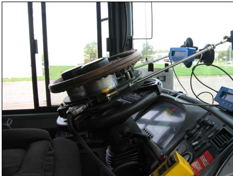
Figure 18. Photo. The steering machine provided repeatable inputs for the high-speed maneuvers.
