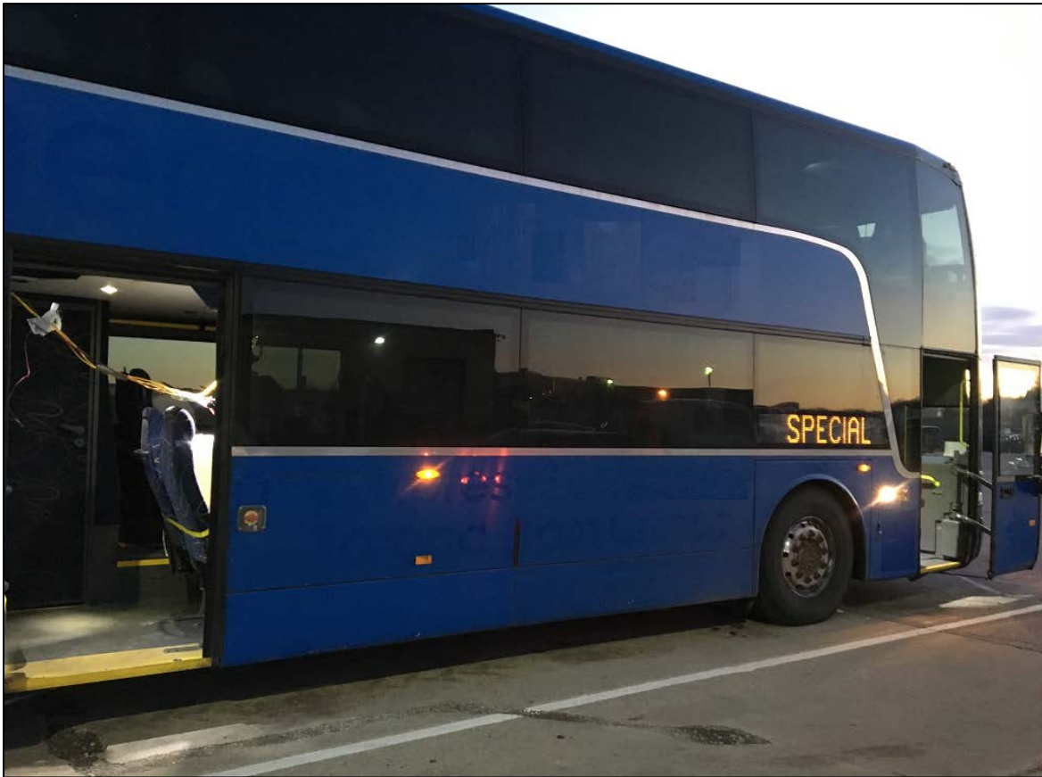
Figure 17. Photo. The motorcoach had doors at the front and rear. It had two stairs, one by each door.
