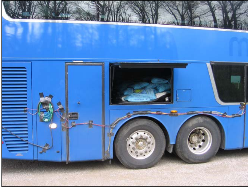
Figure 6. Photo. Salt bags in the luggage compartment in the vehicle, which is aft of the lower deck seating.
