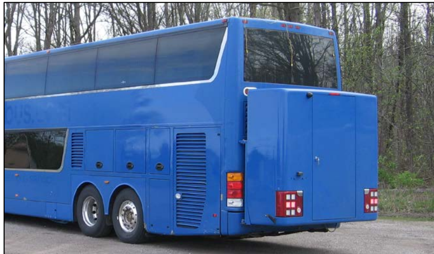
Figure 2. Photo. The rear luggage compartment extends the length of the motorcoach by about 2 ft, 11 in.
