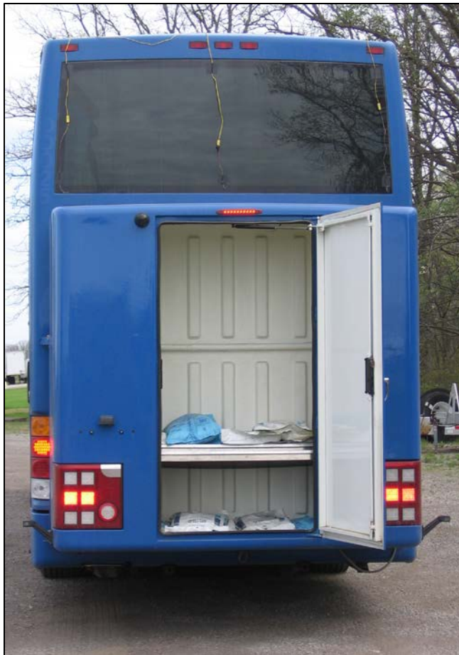
Figure 7. Photo. Bags of salt were distributed on shelves of the rear luggage compartment.
