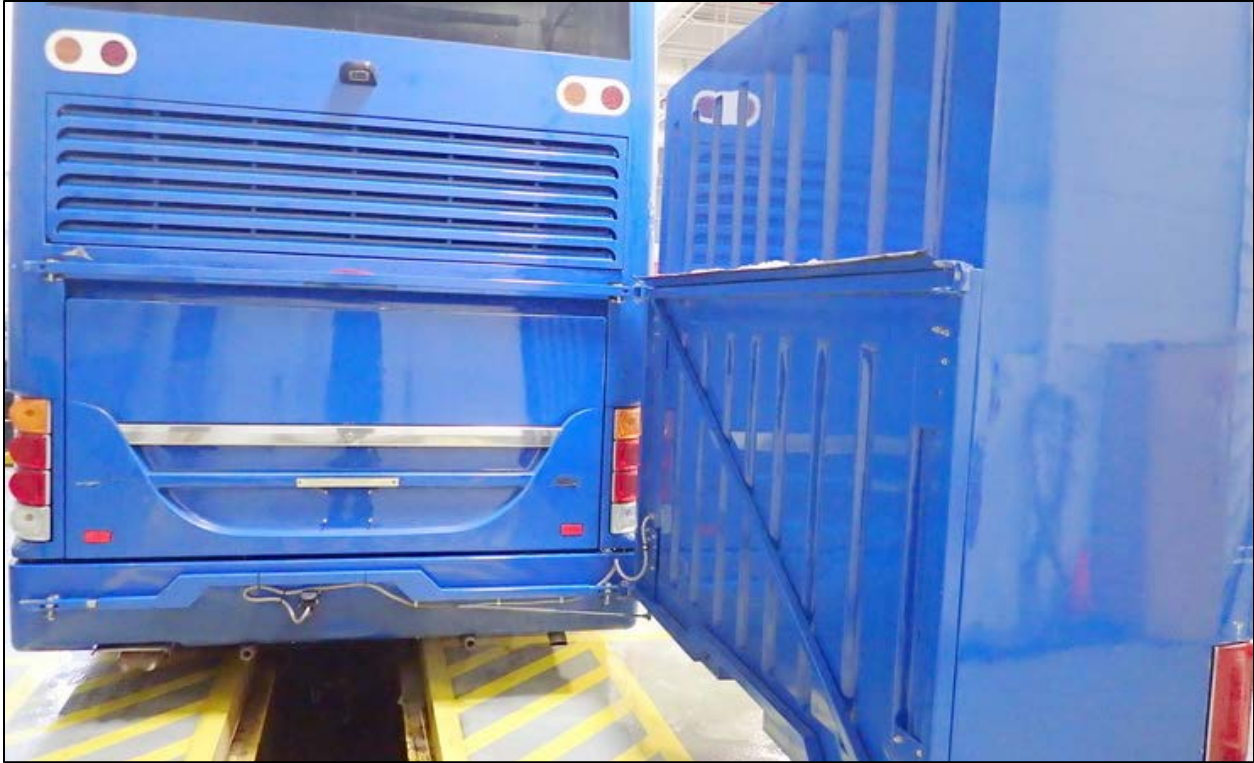
Figure 4. Photo. The luggage compartment can swing away from the motorcoach.
