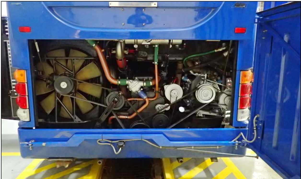
Figure 12. Photo. The engine compartment was accessible after the luggage compartment (visible at the right) was swung out of the way and a door was lifted.
