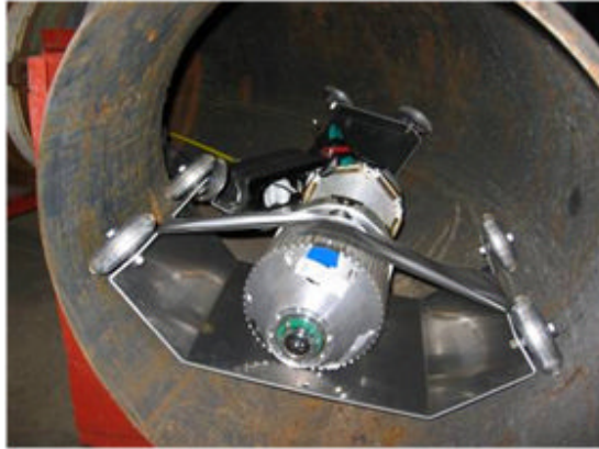
Figure 5.5.1.2: Vehicle built for wireless test at NYSEARCH Test Bed
