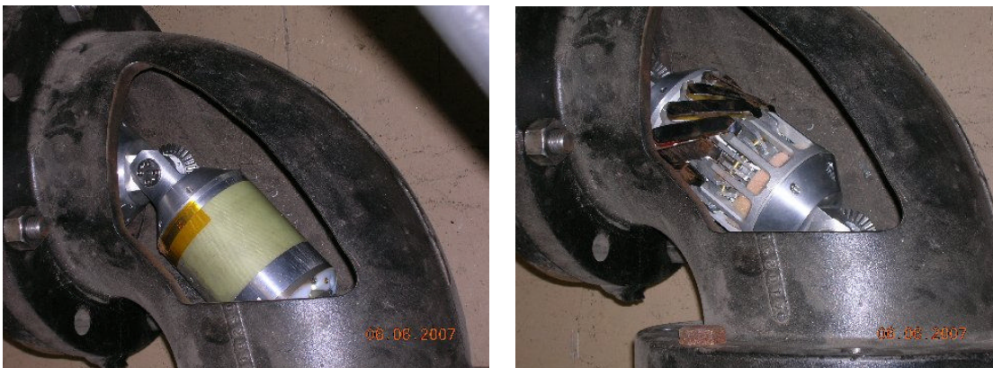
Figure 5.2.2: Excitation coil module and sensor module negotiation a 90-deg bend.
