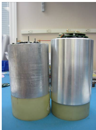
Figure 5.5.2.3: An original Explorer II battery module (left) and a new, higher capacity battery module (right). (Yellow ring on bottom of both modules is for support and is not part of the module.)
