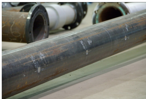
Figure 5.2.3: Sample of defects manufactured on pipes
