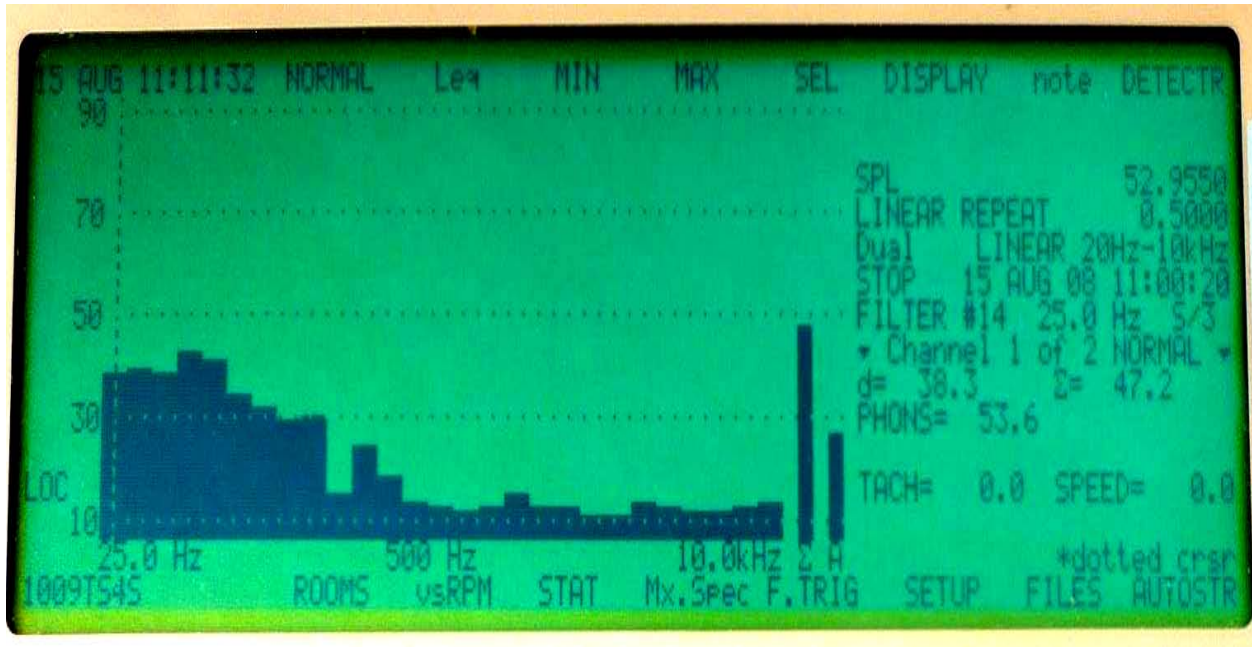
Figure 5. Photograph of the display of a one-third-octave-band analysis of the self-generated noise of a DUT with 16 bit resolution and 44.1 kHz sampling frequency.
