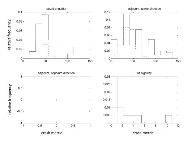
Figure 8.5 Effect of LDW on Frequency Distributions for Component Crash Metrics (Right lane, Scenario 1, Rural). Solid: without LDW, dashed: with LDW.
