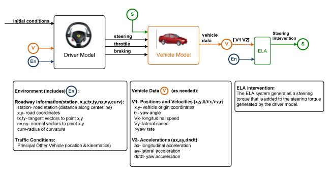
Figure D.5. ELA Functionality Added to the DVET Model
