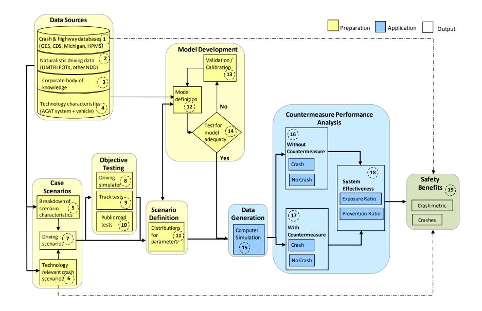
Figure 2.1. Overview of the SIM Components
