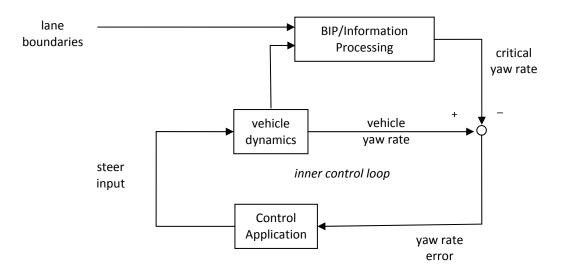
Figure C.2. Structure of the Driver Model Control Loops Used in Parameter Estimation
