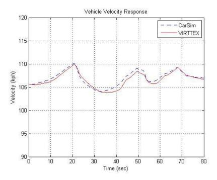
Figure 6.8. Vehicle Model Velocity Responses to Identical Driver inputs
