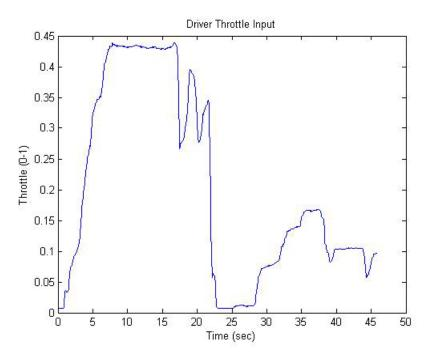
Figure 6.6. Throttle Input From the Driver During the Period of High Longitudinal Acceleration
