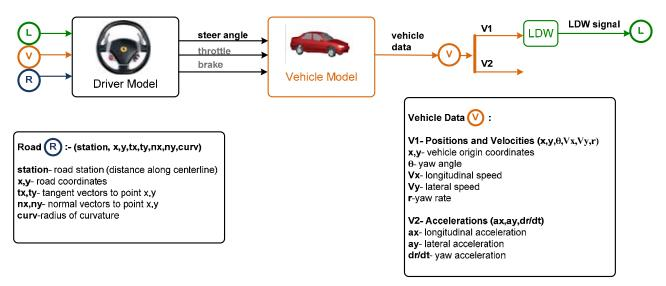
Figure 6.1. Architecture of the Coupled Vehicle-Highway-Driver Model
