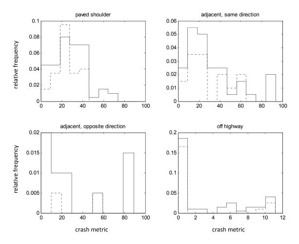
Figure 8.6 Effect of LDW on Frequency Distributions for Component Crash Metrics (Right lane, Scenario 2, Rural). Solid: without LDW, dashed: with LDW.
