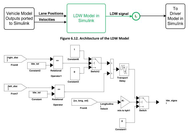
Figure 6.13. LDW System Sub-Model in Simulink
