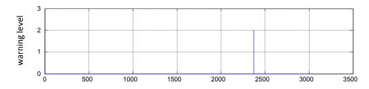
Figure D.2. Time History of DAC Warning Signal (0 = off, 1 = left side warning, 2 = right side warning)
