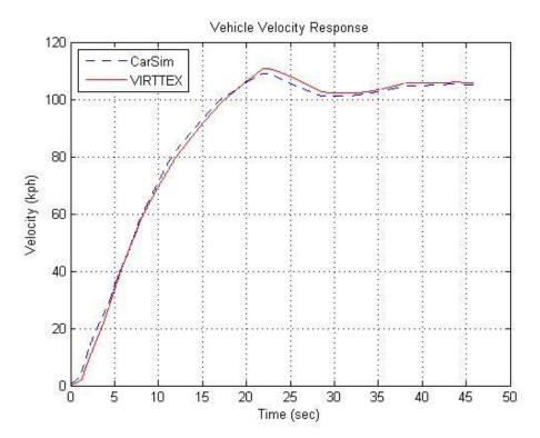
Figure 6.5. Vehicle Model Velocity Response to the Same Throttle Input
