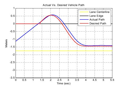
Figure D.8. Actual and Desired Vehicle Path for ELA Activation
