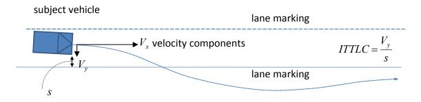
**Figure 7.2.** Inverse Time to Lane Crossing (ITTLC). Note: *s* is the distance between the outside of the leading front tire and the inner edge of the nearest lane line marker, shown here for lateral drift towards the right lane edge.
