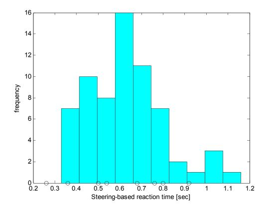
Figure C.10. Reaction Times  $RT_{S0}$  of 40 Simulations (histogram) and VIRTTEX Sleep Deprived Driver Reaction Times  $RT_S$  (circles).
