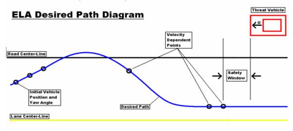
Figure D.4. Schematic of ELA Operation
