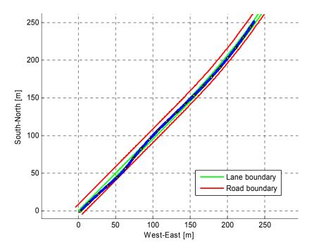
Figure 8.18. Simulation Run for DS 10 Crash Event (LDW=ON)
