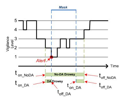
Figure D.3. DAC Exposure Effect: Estimated Reduction in "Drowsy Driving Time"
