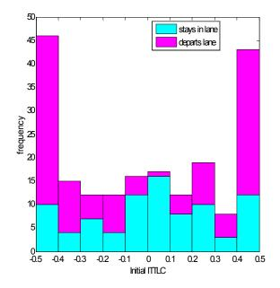
Figure 8.1. Distribution of Initial ITTLC Values (Scenario 1, four lane divided highway, rural locations, right travel lane). Note the extreme bins actually cover a wider ITTLC range than shown
