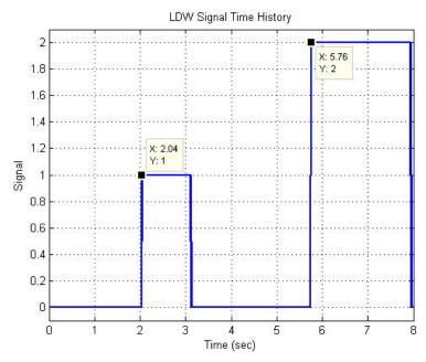
Figure 6.14. Time Periods of LDW Signal Activation [0: no warning, 1: left side warning, 2: right side warning]
