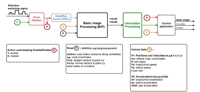
Figure 6.18. Driver Model: Overall Architecture
