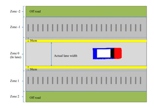
Figure 7.5. Zones for Simulation Control and Crash Metric Analysis.
