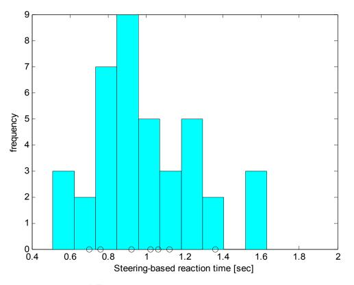
Figure C.9. Reaction Times  $RT_{S0}$  of 40 Simulations (histogram) and VIRTTEX Distracted-Driver Reaction Times  $RT_{S}$  (circles).
