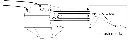
Figure 4.1. Driving Scenario Resolution for Monte Carlo Simulation - With and Without the Specific Safety Technology Being Evaluated.
