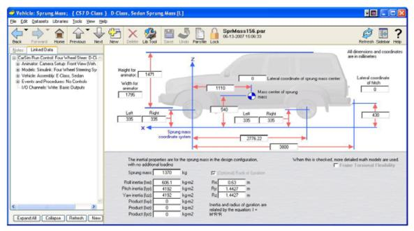
Figure 6.3(b). CarSim Screenshot: Vehicle Sprung Mass Parameters.
