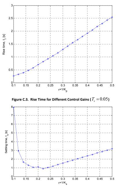
Figure C.4. Settling Time for Different Control Gains ( $T_s = 0.05$ )
