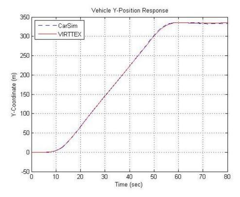
Figure 6.10. Vehicle Model Y-coordinate Responses to Identical Driver Inputs.
