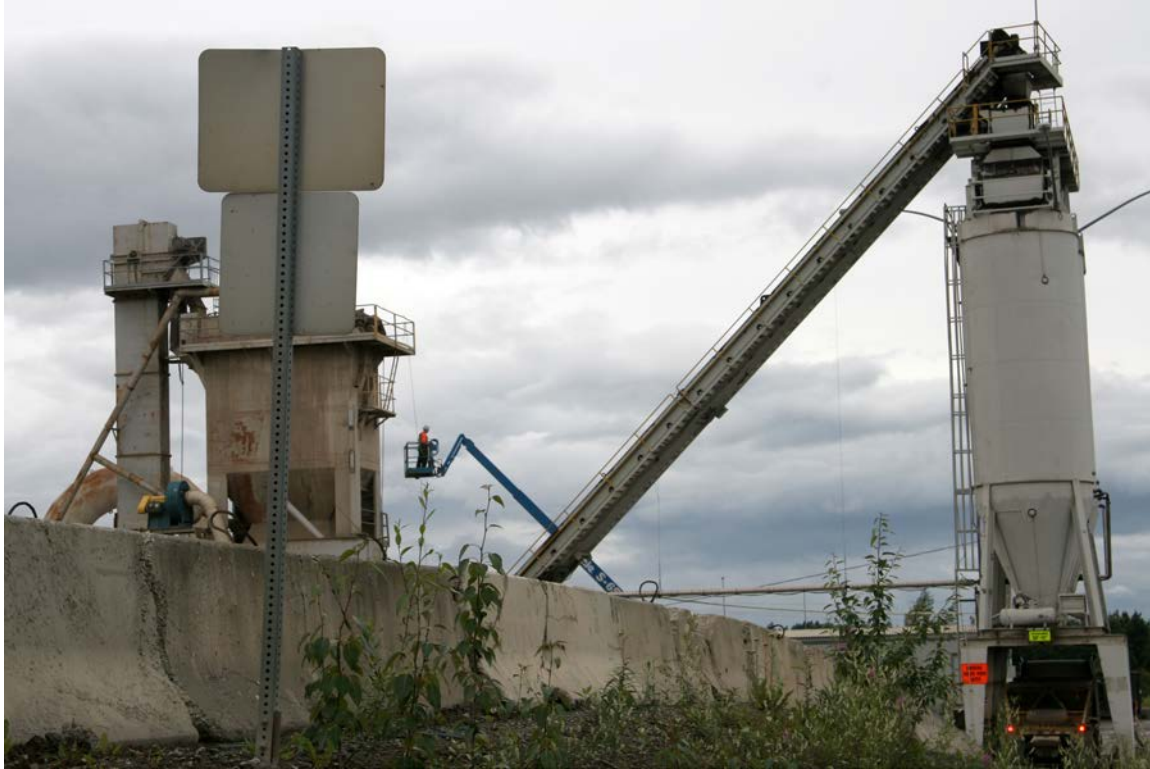
Figure 5.3: Stationary asphalt plant off Dowling Road in Anchorage, showing truck loading to the far right. Photo by Janet Burton, University of Alaska.
