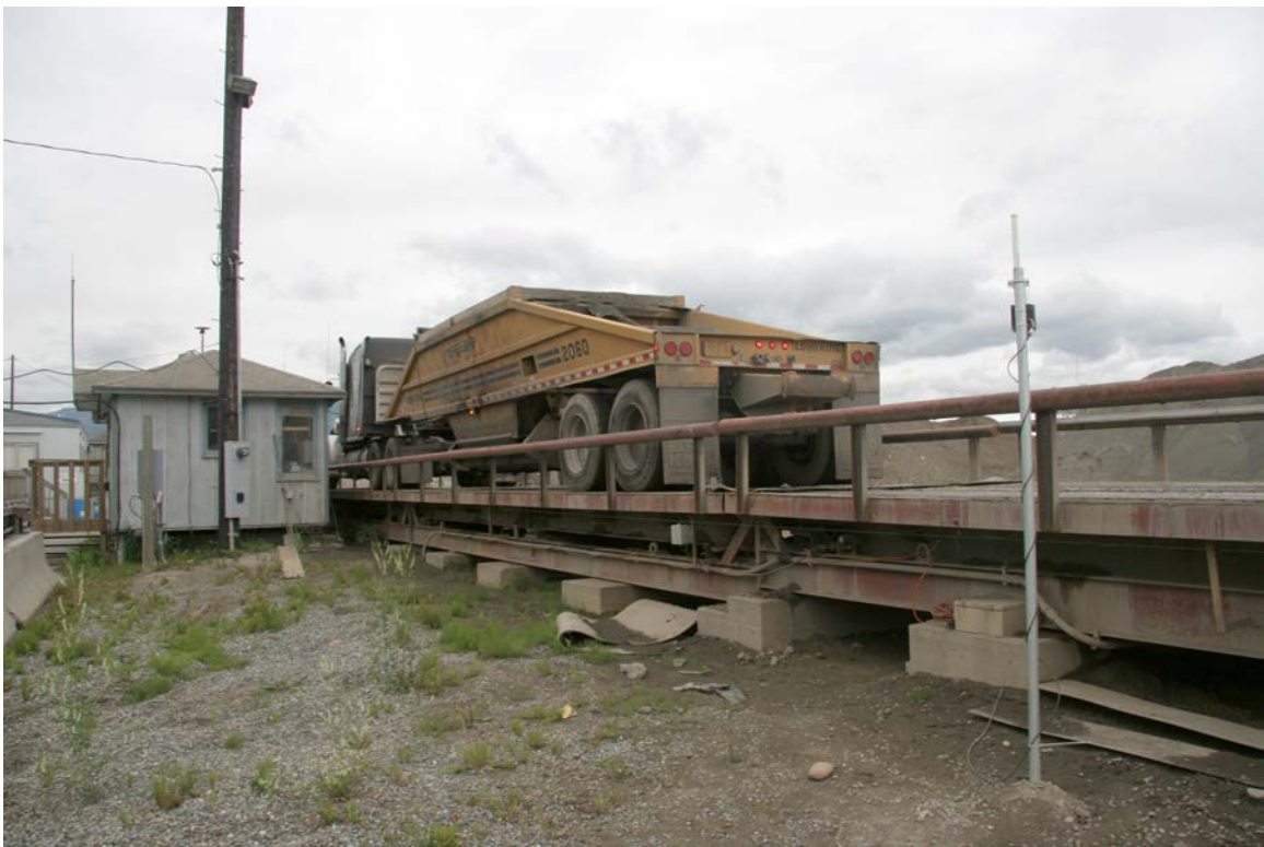
Figure 5.1: Granite scale in Anchorage with stationary pole and RFID reader/antenna in the foreground. The PaveTag™ processing hardware is the gray box sitting on top of the concrete support, next to the antenna pole. Photo by Janet Burton, University of Alaska.
