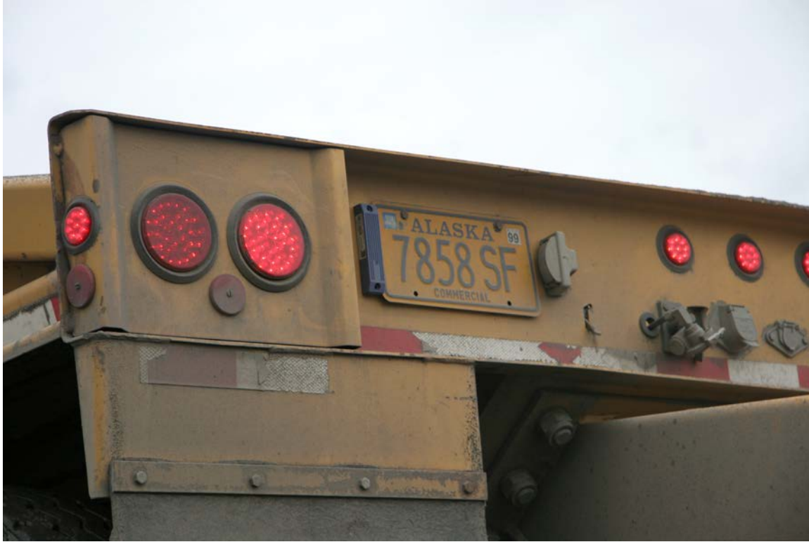
Figure 5.2: RFID tag mounted to the left of the license plate.
