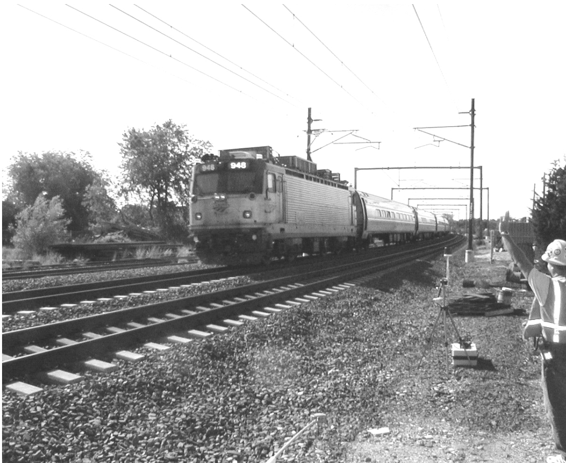
Figure K1. Photograph of Passing Northbound Regional Train (third measured pass). The RF Probe Mounted on a Tripod is Visible just beyond the Flagman
