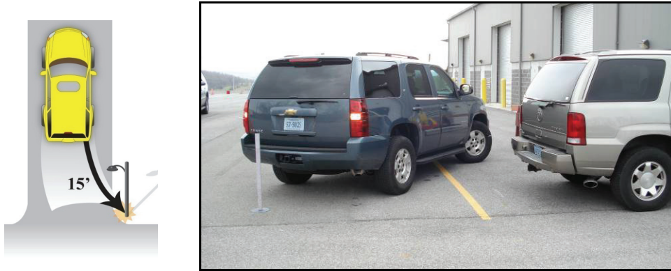
Figure 106. Vehicle Scenario 10: Intermediate Static Pole, as Conceptualized (Left) and Realized (Right)
