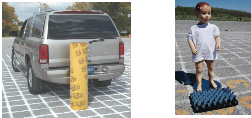
Figure 33. Grid Test objects used to assess camera Field Of View (FOV)
