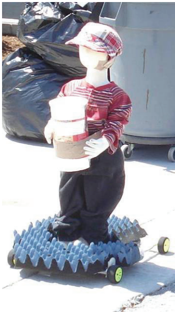
Figure 31. Movement platforms used for Grid Tests (Left) and Driver-in-the-Loop Tests (center & right)
