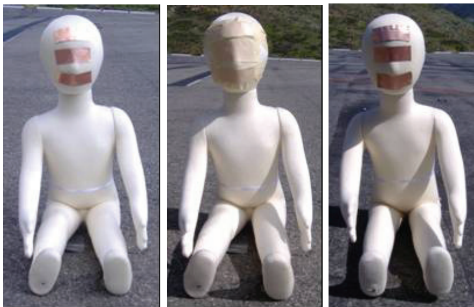
Figure 11 - Seated two-year-old child mannequins, from left to right: FLEX-2T-seated-A, FLEX-2T-seated-A with masking tape, and FLEX-2T-seated-B. FLEX-2T-seated-B with masking tape is not shown
