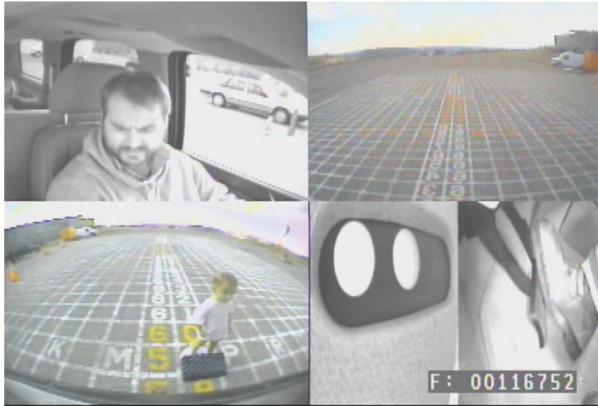
Figure 37. Video instrumentation excerpt for static field of response trial with standing 2-year-old mannequin. LED display (lower right quadrant) indicates a response.
