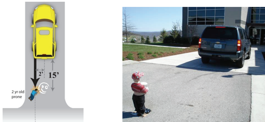
Figure 76. Pedestrian Scenario 3: Intermediate, Static Pedestrian, as Conceptualized (Left) and Realized (Right)
