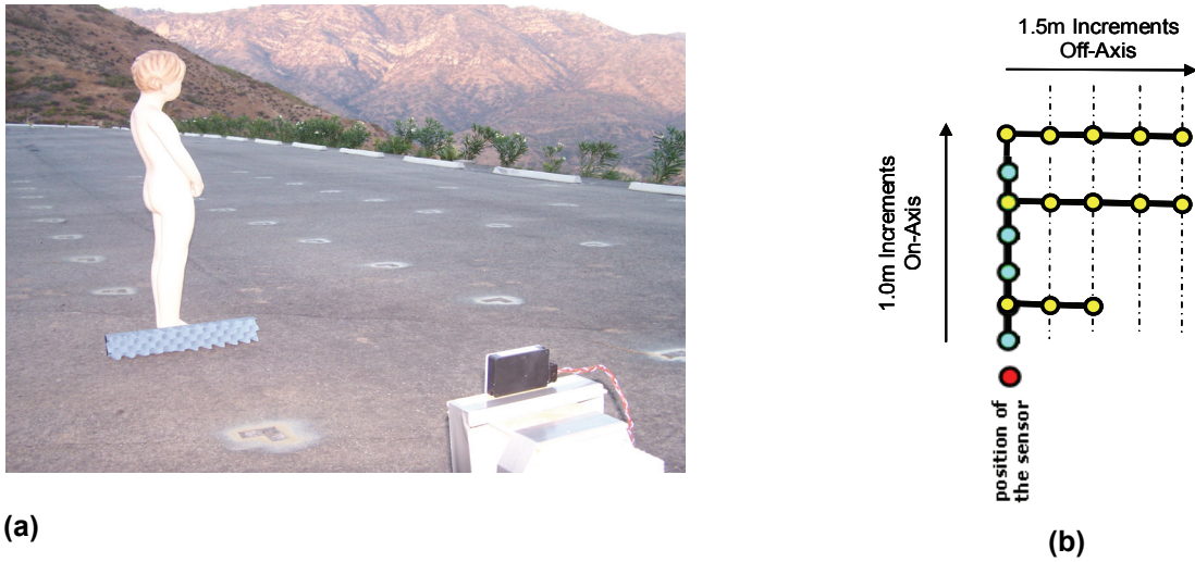
Figure 4. HRL's outdoor radar test setup (a) and grid (b).
