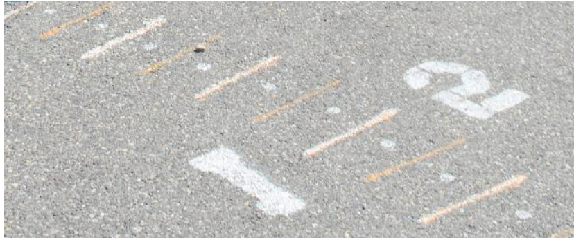
Figure 29. Circular Test Grid showing 3” scaled units
