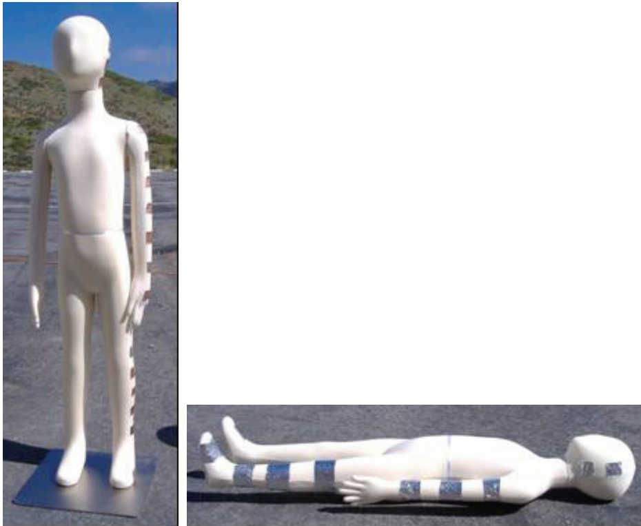
Figure 9 - Five-year-old child mannequins modified for the supine posture, from left to right: FLEX-5-supine-A (shown standing upright) and FLEX-5-supine-B. FLEX-5-supine-A also serves the role of a five-year-old in the standing posture (i.e. FLEX-5-standing-B).
