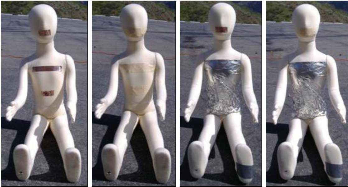
Figure 8 - Seated five-year-old child mannequins, from left to right: FLEX-5-seated-A, FLEX-5-seated-A with masking tape, FLEX-5-seated-B, and FLEX-5-seated-B with masking tape)
