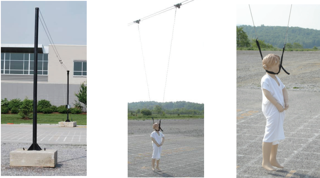
Figure 42. Method of suspending and moving test objects over the Test Grid
