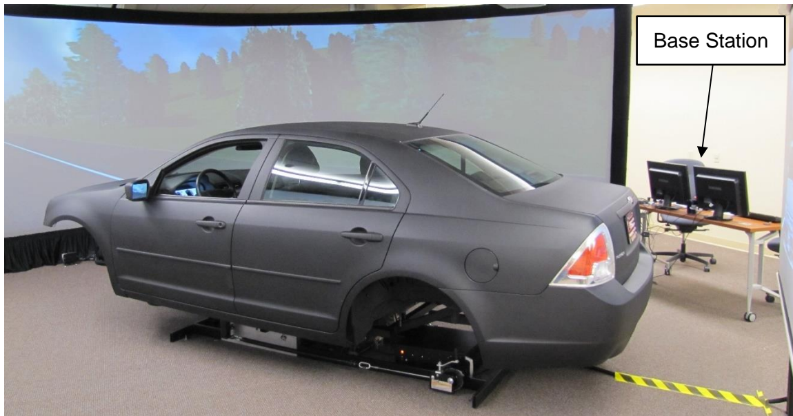
Figure 5.3 UW-Madison Driving Simulator
