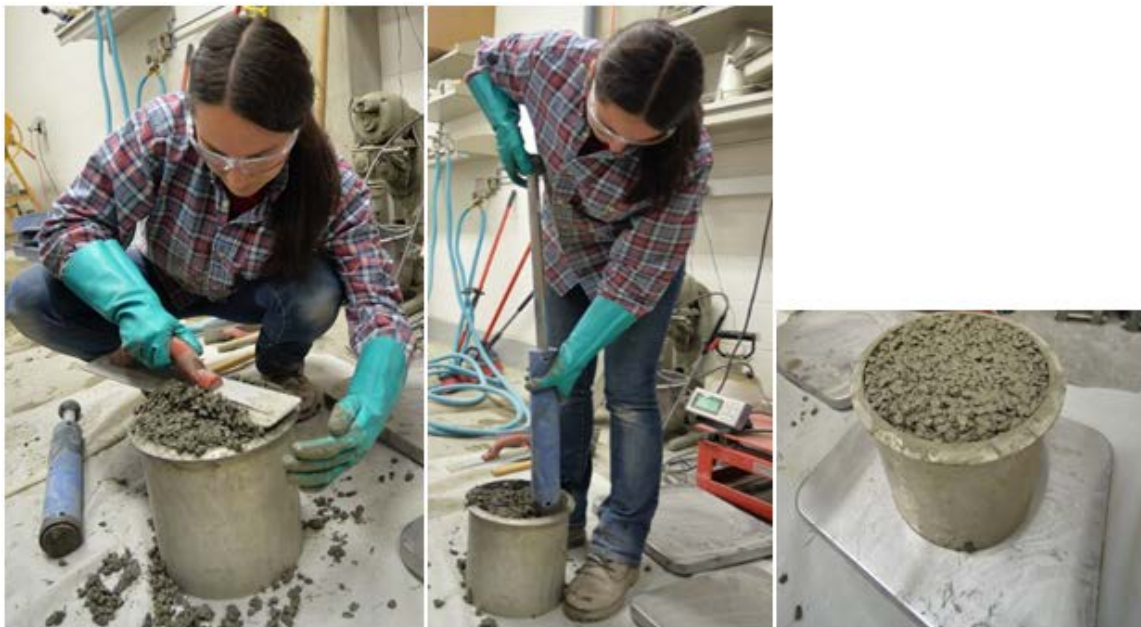
Figure 4. Photos show the process to establish fresh density of PC
