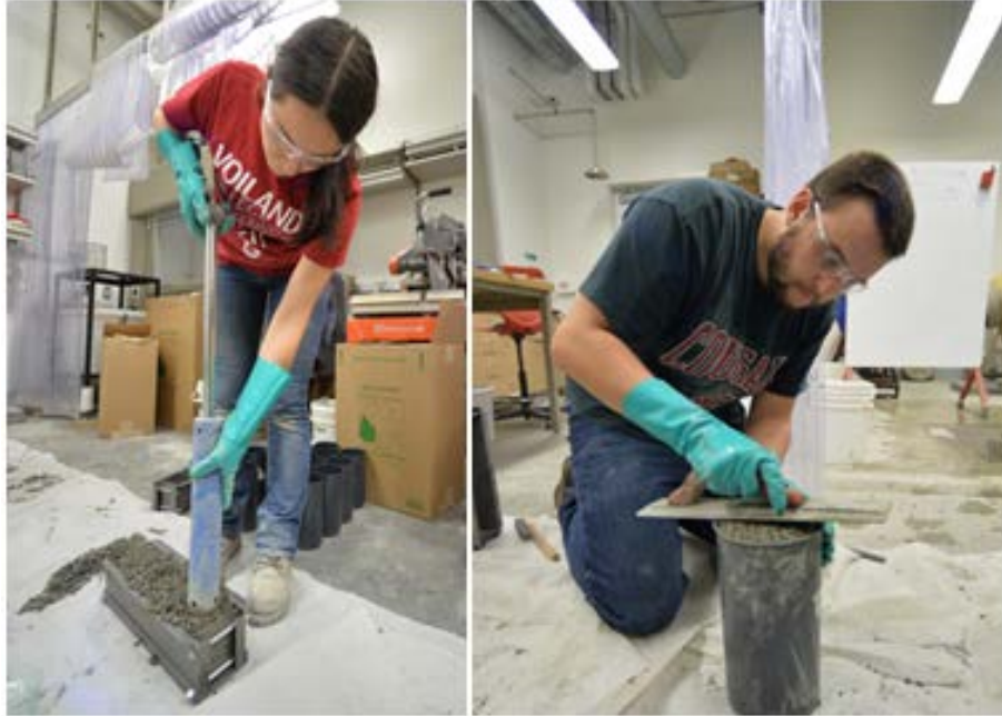
Figure 5. Photo on the left: using proctor hammer to compact PC specimen, photo on the right: finishing PC specimens using a float
