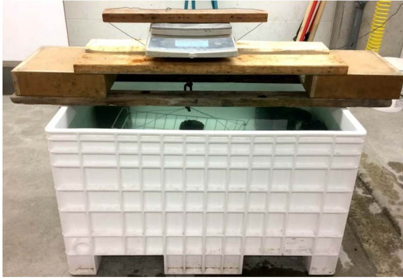
Figure 6. Hardened porosity test setup where the mass of submerged PC specimen is measured
