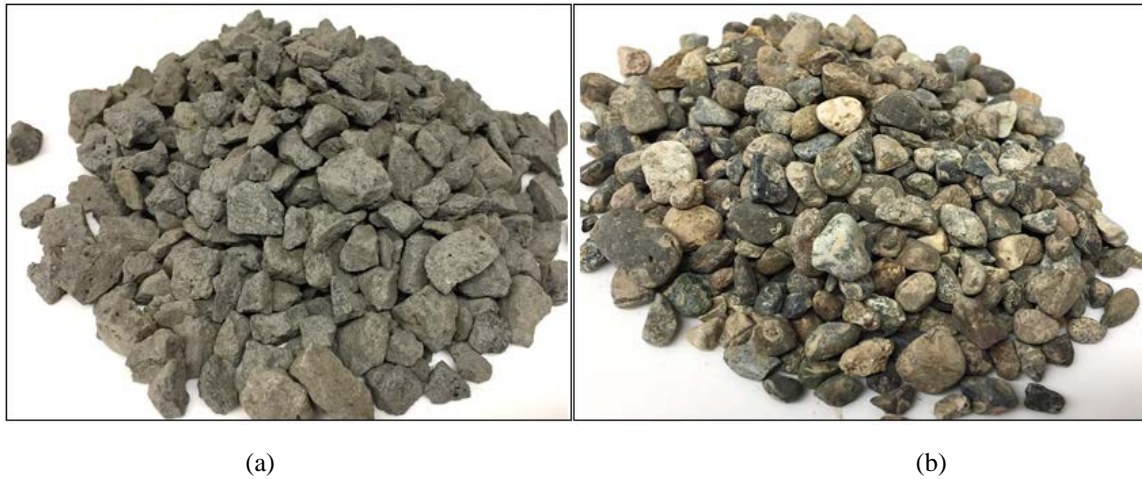
Figure 2. Photos of samples from the (a) crushed basalt; (b) pea gravel aggregates used in the study
