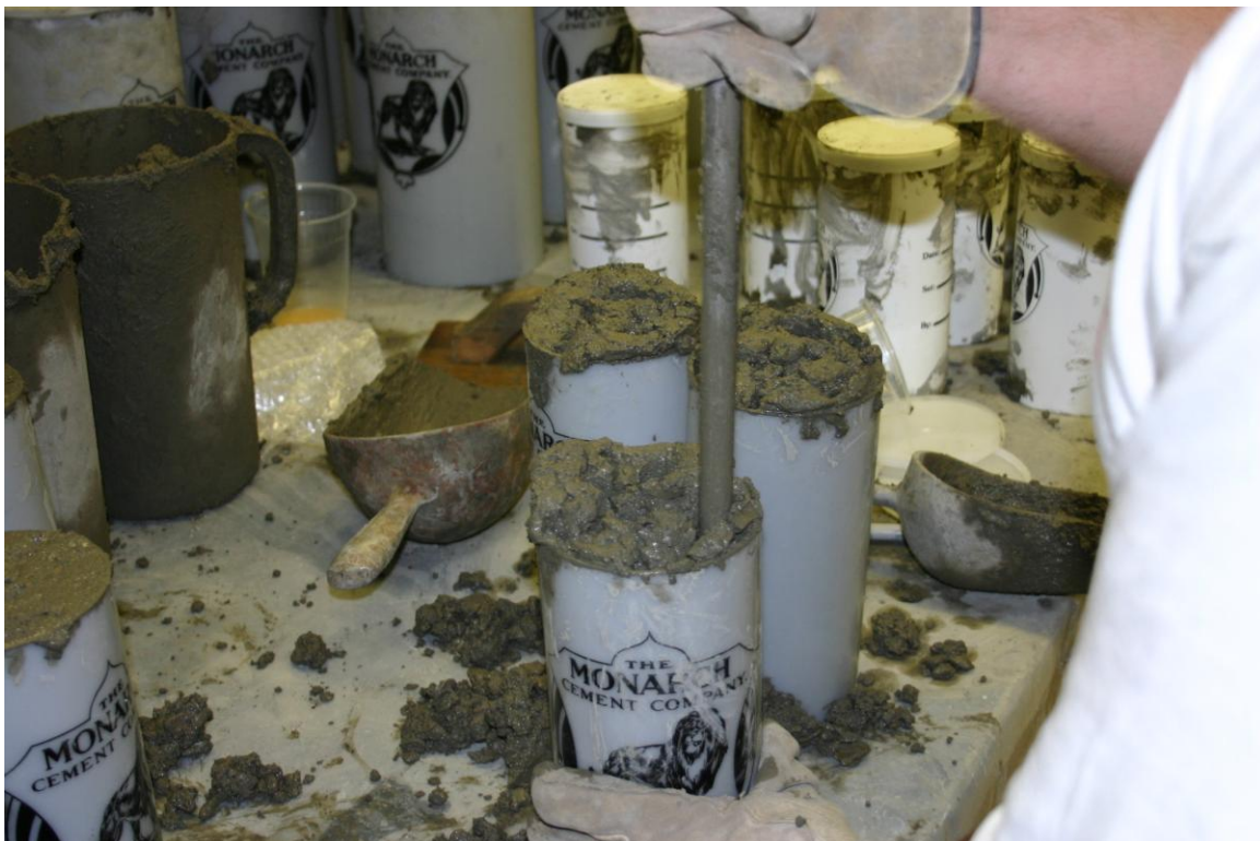
Figure 18. Making concrete cylinders.
