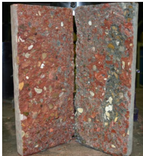
Figure 32. Core after split-tensile test.
