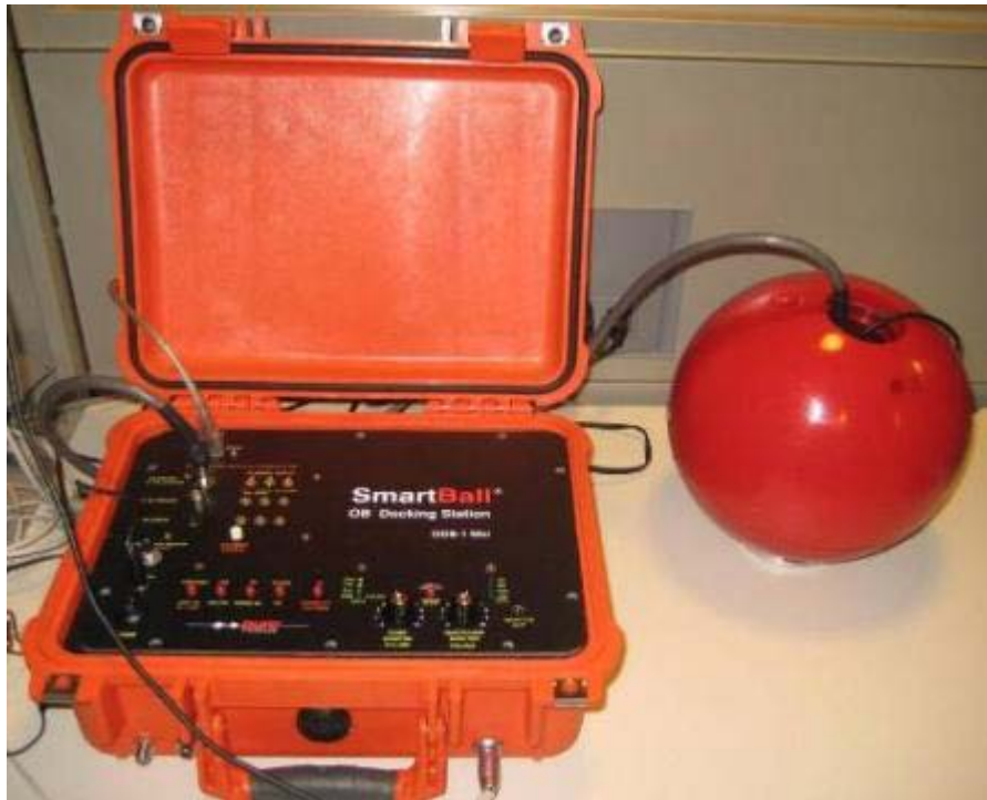
Figure 12. SmartBall Docking Station for Direct Uploading of Captured Data
