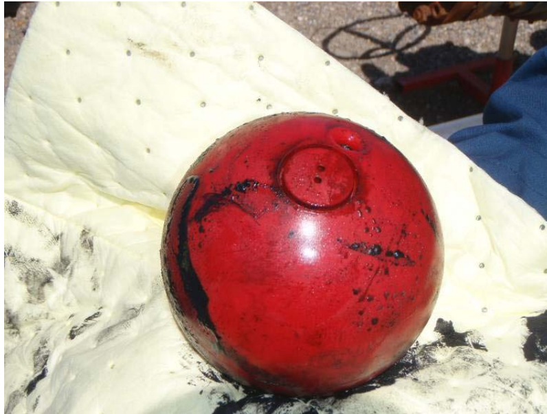
Oilball after Crude Oil Pipeline Inspection
