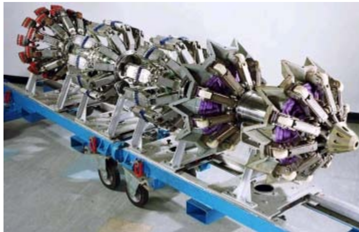
Figure 8. Traditional In-Line Inspection Tool
