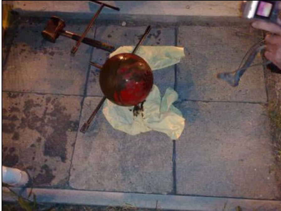
Figure 21. The 10" OilBall Removed from Pipeline
