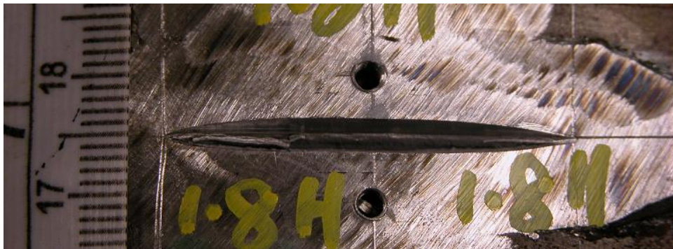
Figure 4-1 Residual flaw opening view from the pipe OD surface after a test
