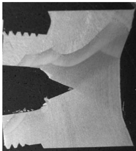
Figure 8-3 Crack-tip profile from a full-scale test specimen
