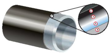
1 Steel 2 FBE 3 FBE/Adhesive Interface 4 Polyethylene
