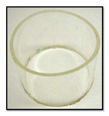
Figure 11 – Typical HPCC Coated Pipe Sample Section
