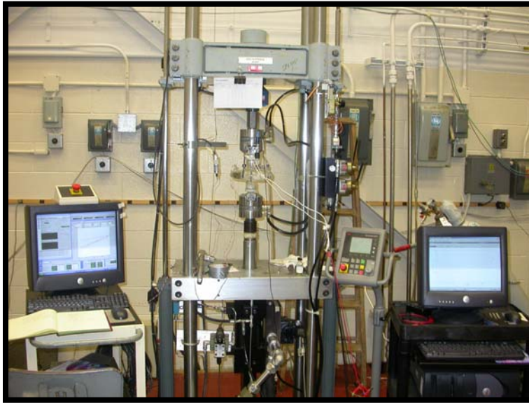
Figure 21. Experimental set up for the NN-pH SCC testing
