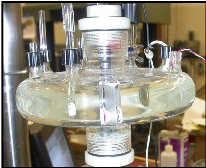
Figure 22. NN-pH SCC test chamber with three electrode system (reference electrode, SCE, and counter electrode, Pt-Au alloy)
