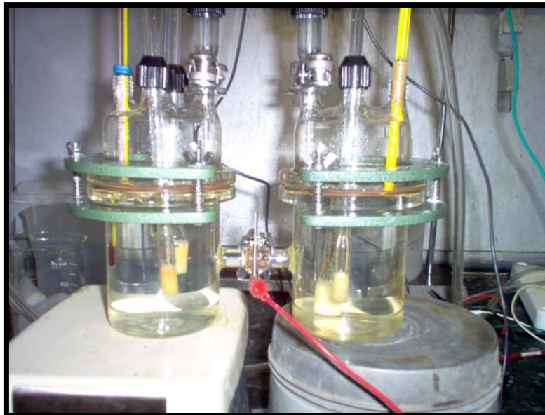
Figure 16. Electrochemical cell for hydrogen permeation experiments through a metallic membrane
