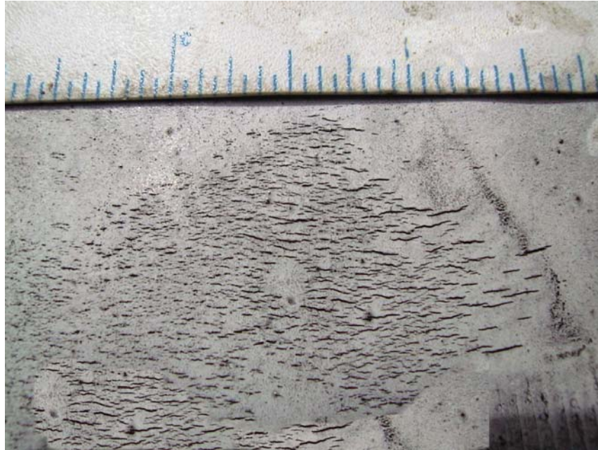
Figure 2 An SCC colony detected using MPI.
