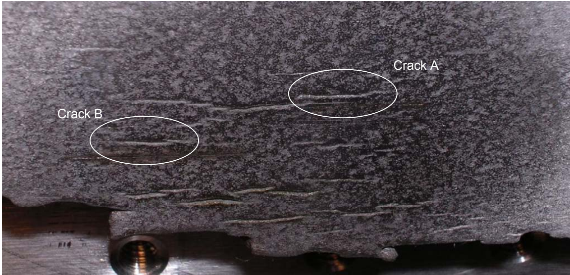
Figure 22 Photo of a portion of the SCC colony in Sample 10409.
