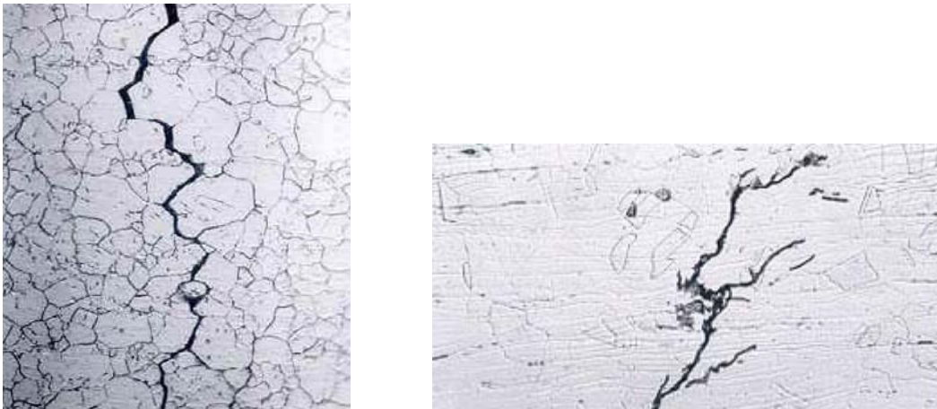
Figure 1 High pH SCC (left) and near neutral SCC (right).
