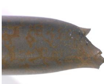
X-70 at the corrosion potential ( \sim -0.7 V)
