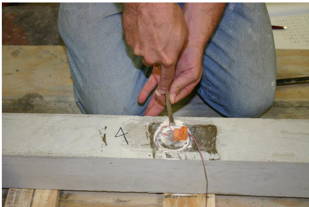
Figure 5.4 Fracturing the core center from the surrounding beam
