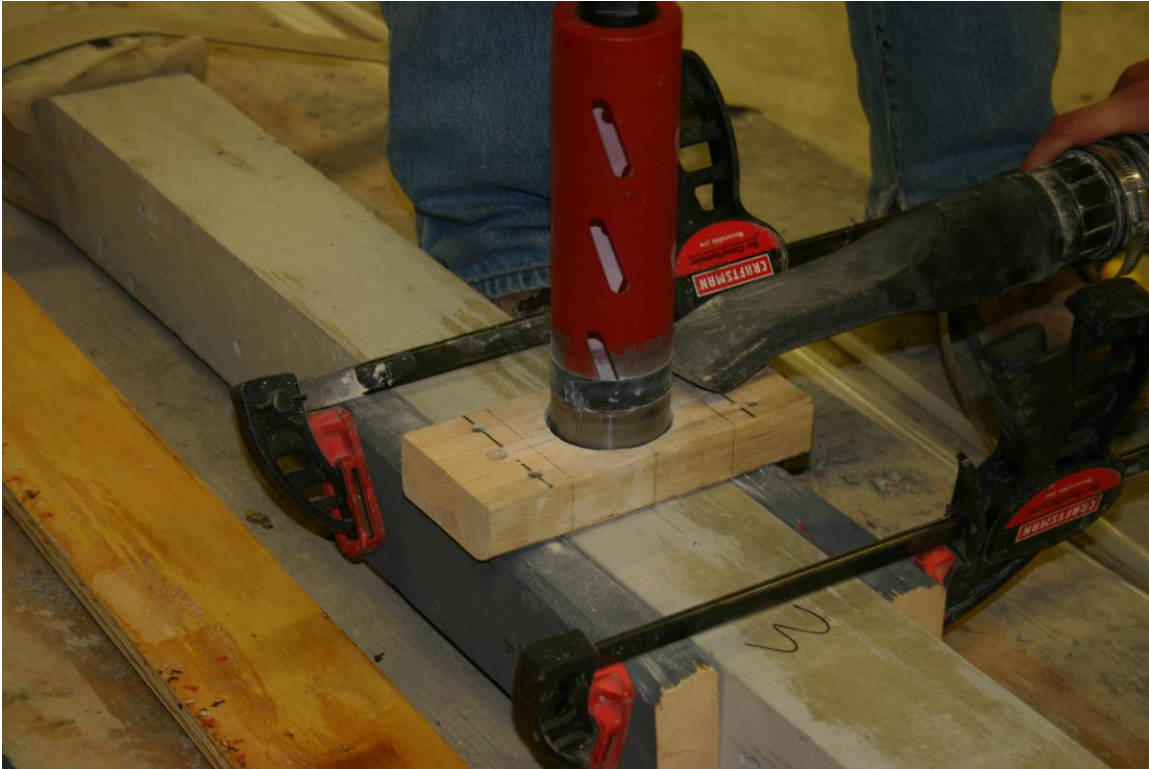
Figure 5.3 Coring the member
