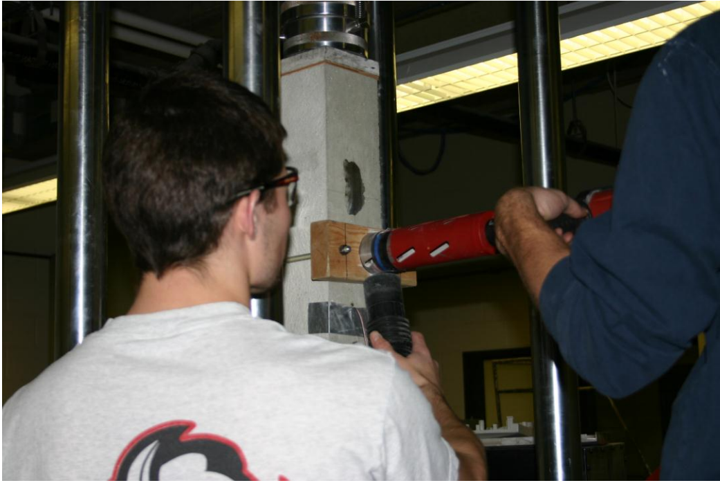
Figure 4.4 Coring around a strain gage
