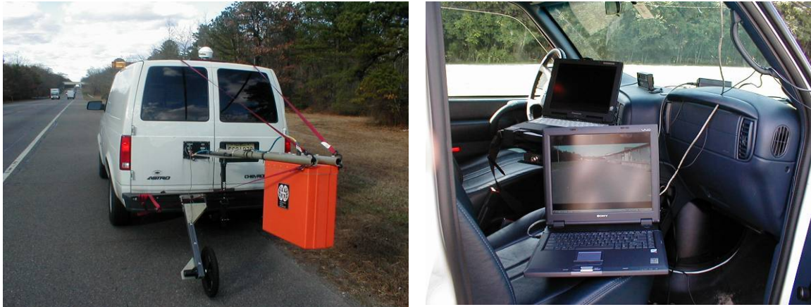
(a) Survey wheel, GPS antenna and GPR antenna
