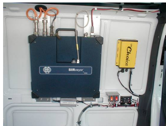
(b) SIR-20 data acquisition unit and GPS Receiver
