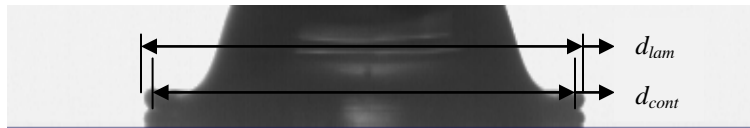
Fig. 2.6 Diameter of the spreading lamella and diameter of the contact line
