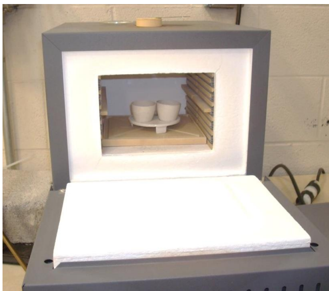
Figure 4: Drying and calcination of customized nickel catalyst using a muffle furnace.
