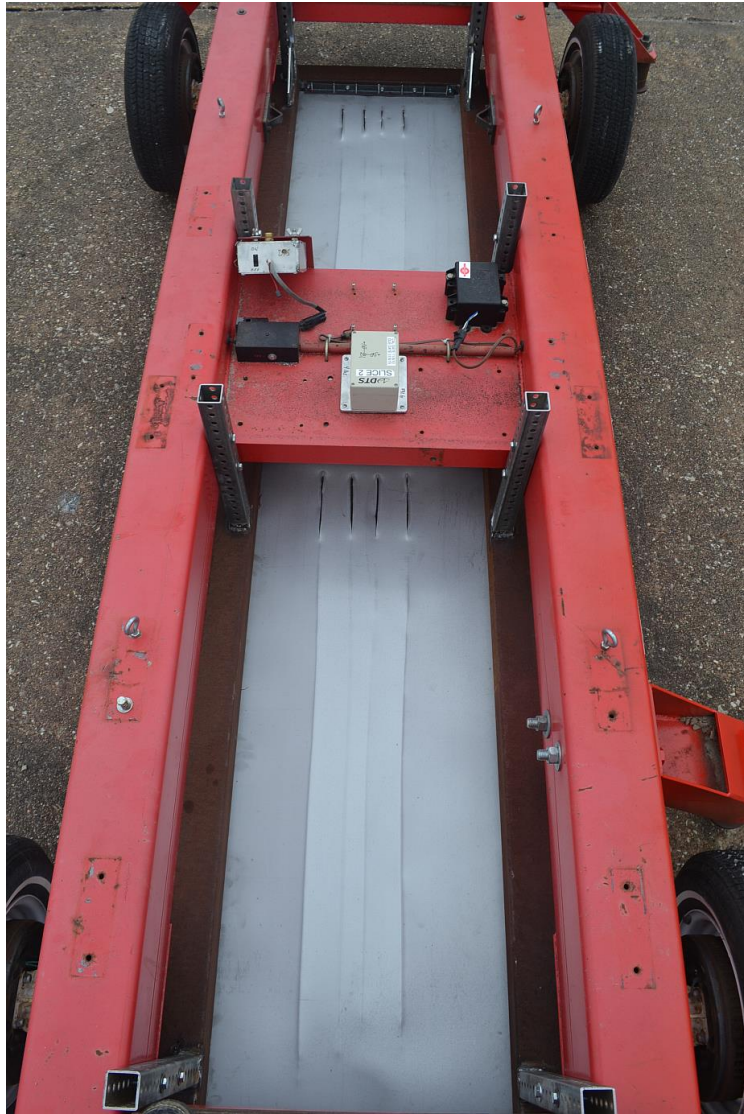
Figure 36. Simulated Floorpan Damage, Test No. MWFPF-4
