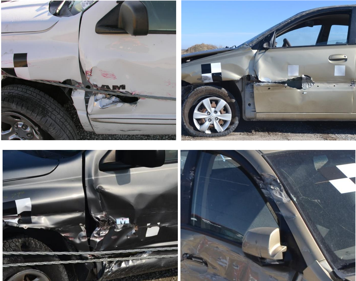
Figure 96: Vehicle Door and A-Pillar Damage from Splice Snagging
