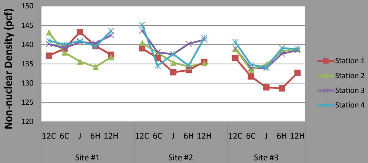
FIGURE 11 Phase 1 PaveTracker Non-Nuclear Density Comparison (pcf).
