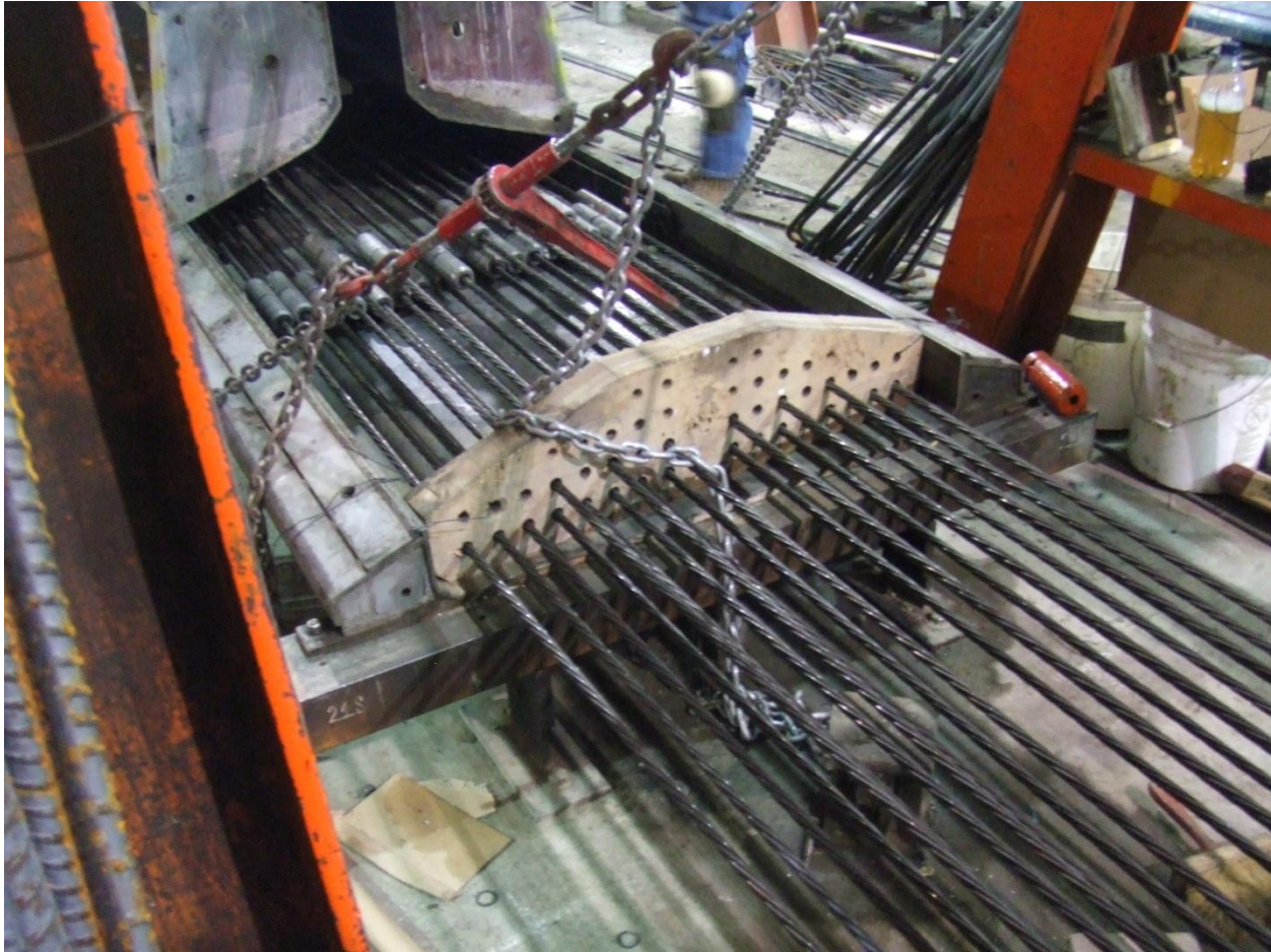
Figure 59. Photo. This strand spacing block is used at the end of the form. Woodworth 2008
