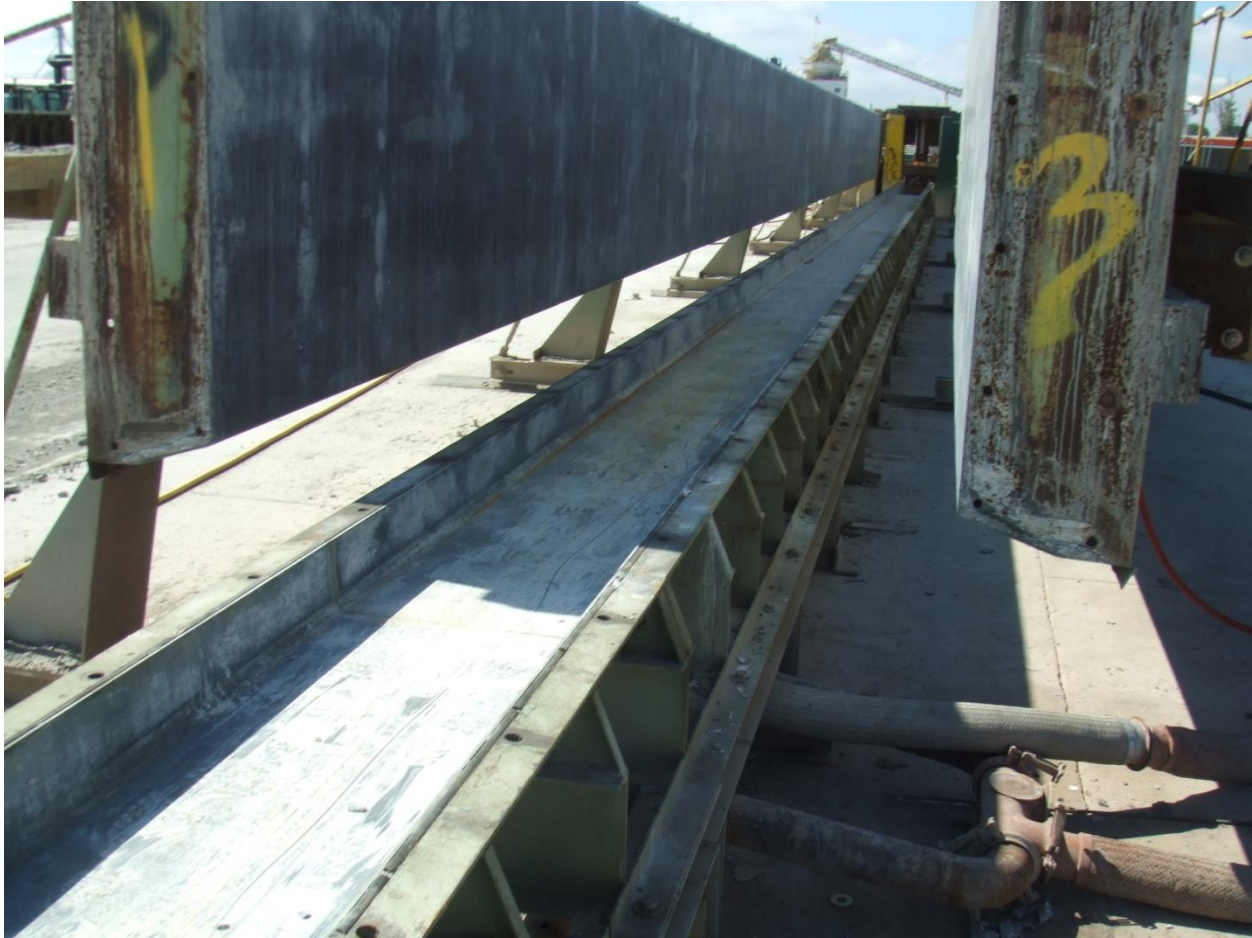
Figure 57. Photo. The bottom soffit pan of this form has bolt holes where the form sides are attached. Woodworth 2008
