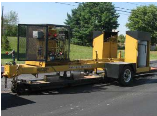
(a) Towed Infrared Heater
