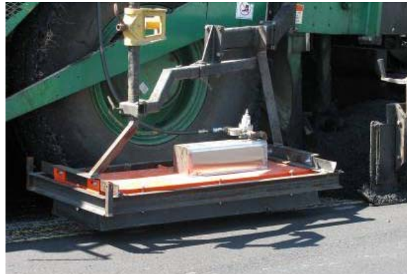
(b) Heater Attached to the Paver
