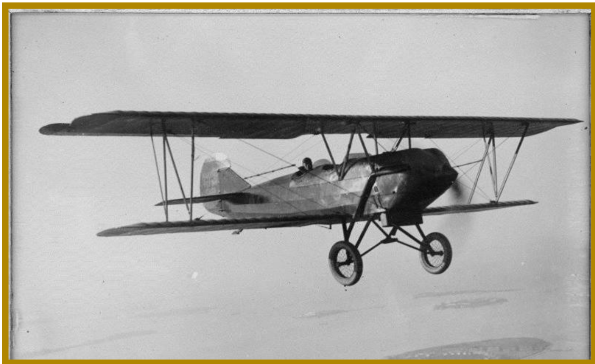
Figure 2.3-4 Travel Air open cockpit biplane with OX-5 engine that was owned and operated by the Harvard Flying Club out of East Boston Airport
