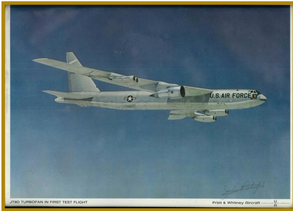
Figure 2.3-7 JT9D engine slung under the wing of a B-52 in its first flight test out of Bradley Field in June 1968
