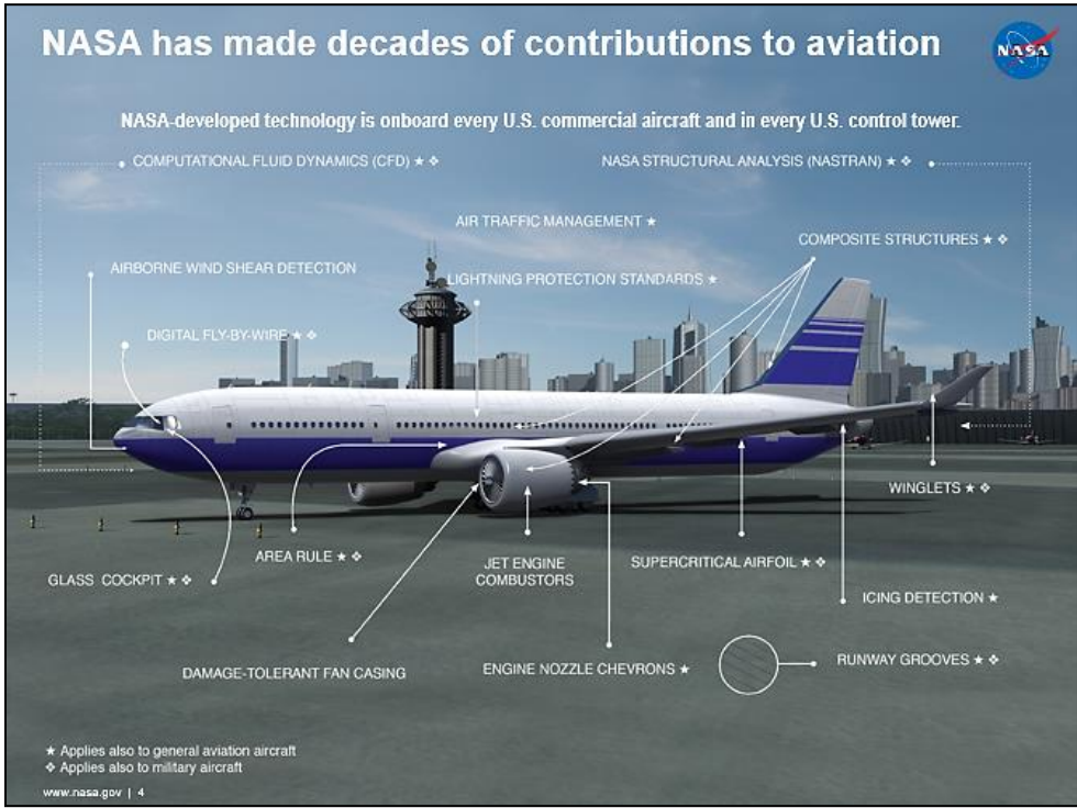
Figure 3.3-3 Examples of NASA's Continuing Contributions to Aviation Technology
