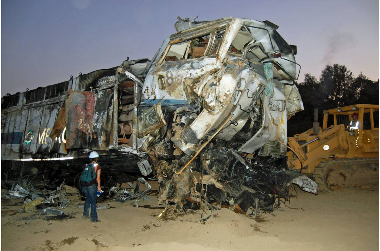
Figure 13. Lead Passenger Locomotive
