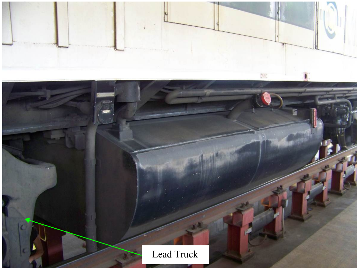
Figure A.3-1. Exemplar Passenger Locomotive Fuel Tank
