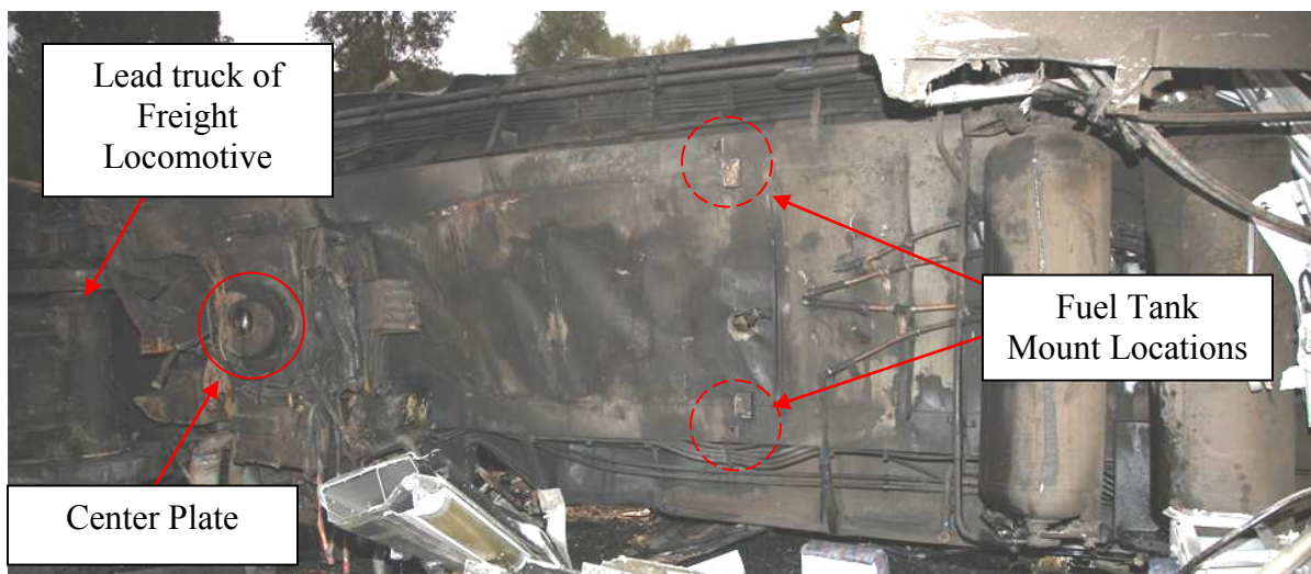
Figure A.3-5. Passenger Locomotive Underframe, Before Locomotive Moved by Rescue and Recovery Crew
