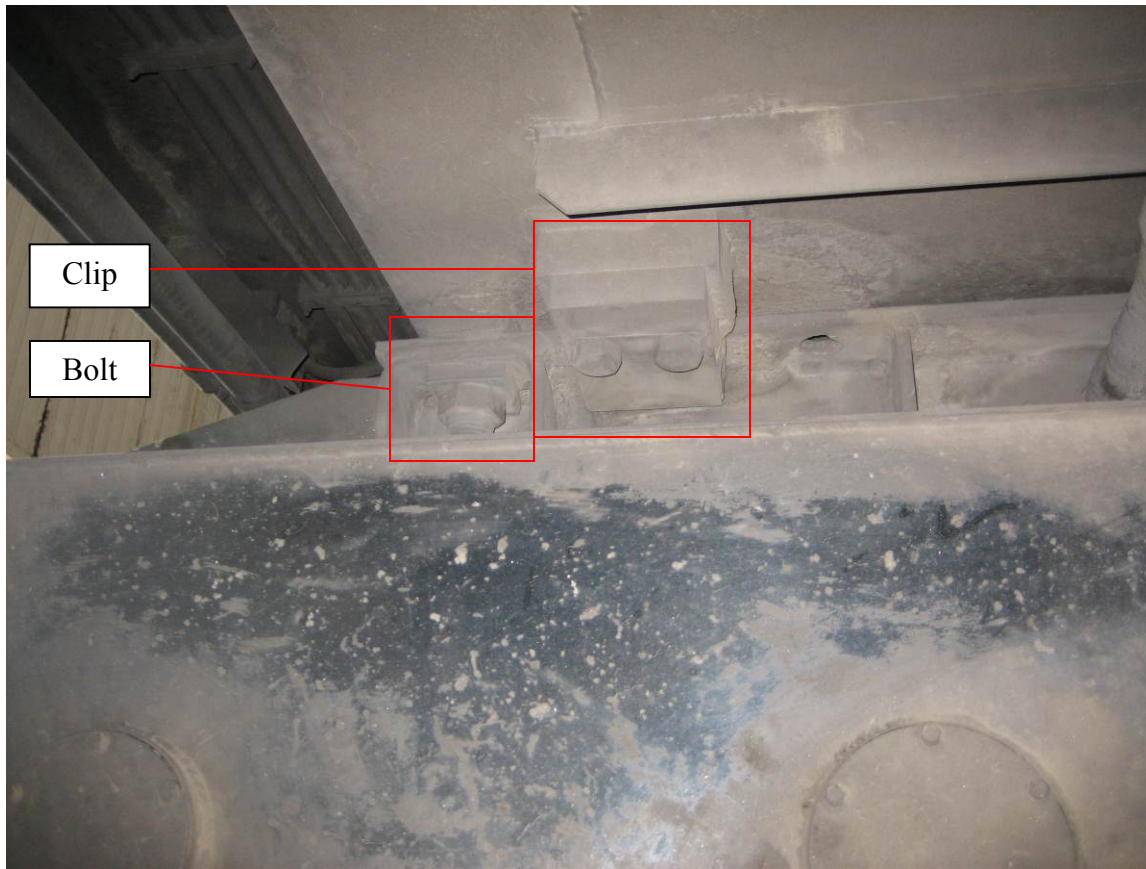
Figure A.3-2. Fuel Tank Attachment to Underframe
