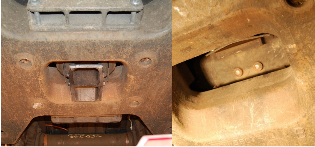
Figure A.2.1-15. Intact Truck Retention Mechanism
