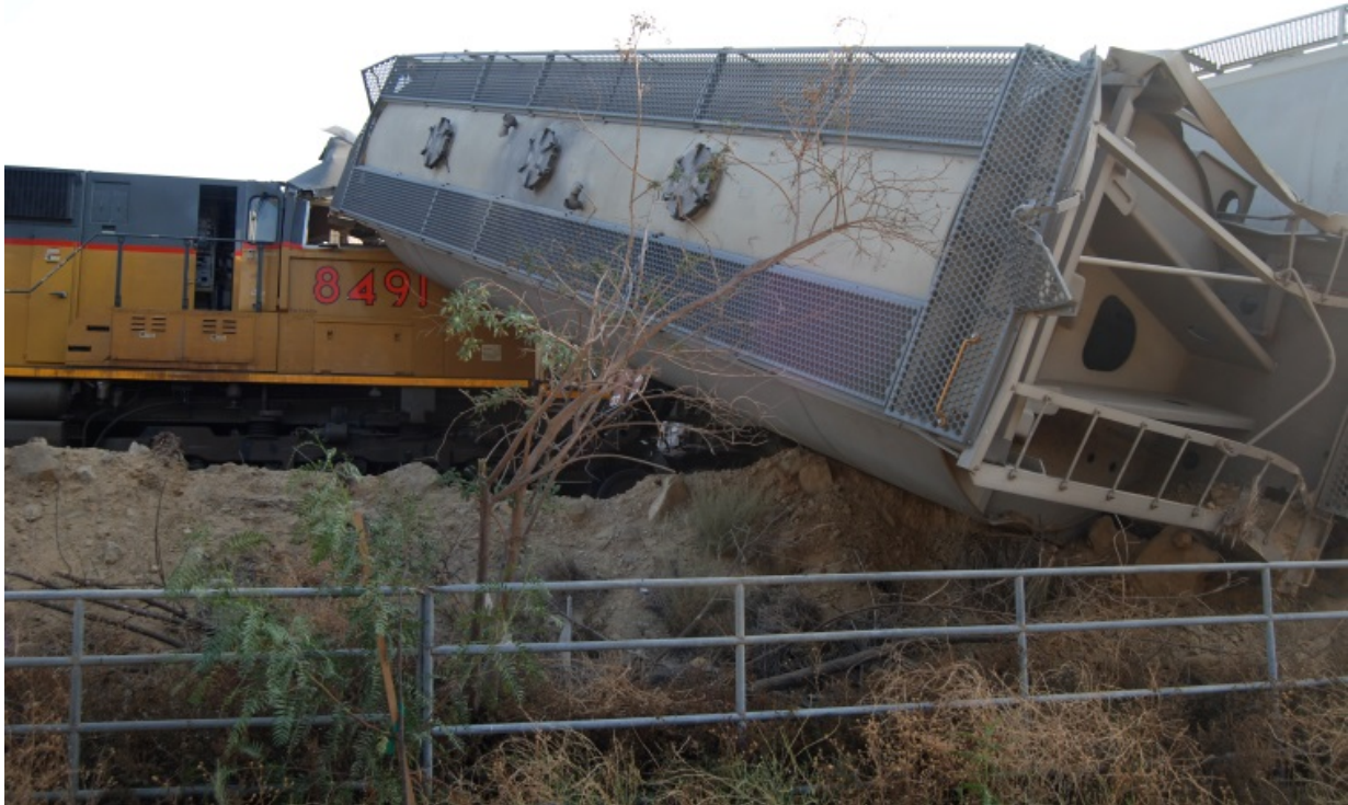
Figure 19b. Second Freight Locomotive Structural Damage
