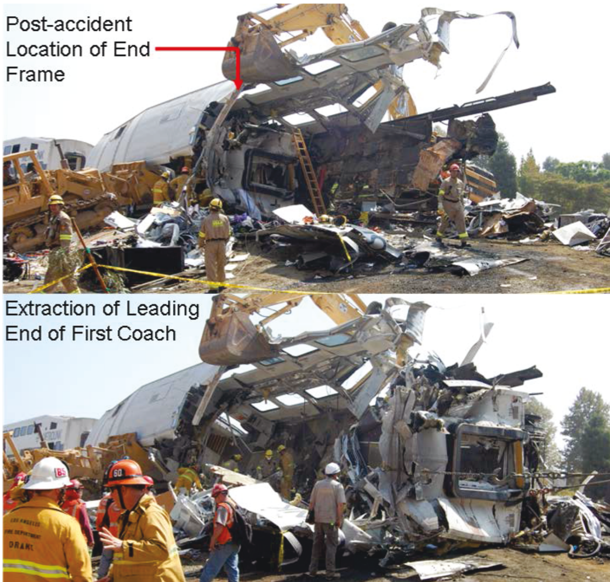
Figure 14. First Passenger Car Structural Damage
