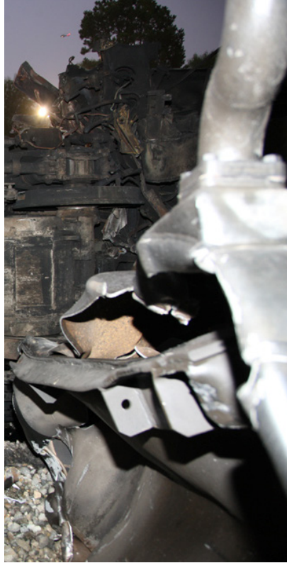
Figure A.3-4. Damage to Fuel Tank Leading End
