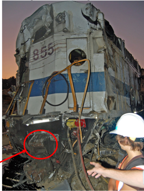
Figure A.1-5. First Passenger Car Lead End Frame Interaction with Locomotive Trailing End Bellmouth
