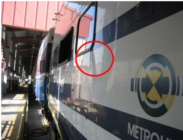
Figure A.2.1-12. Second Passenger Car Sidewall and Truck Attachment Damage
