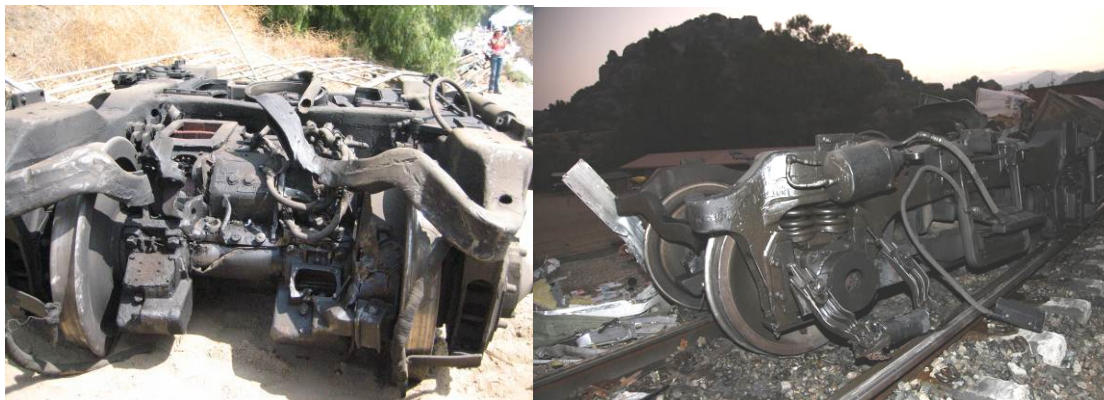
Figure A.3-9. Passenger Locomotive Lead Truck: Leading End (left) and Trailing End (right)
