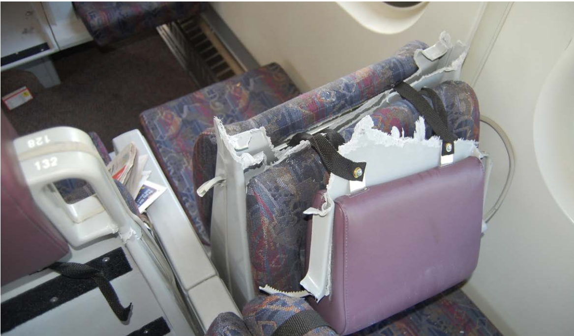
Figure 23. Broken Head Rests in Lower Level, Car #617
