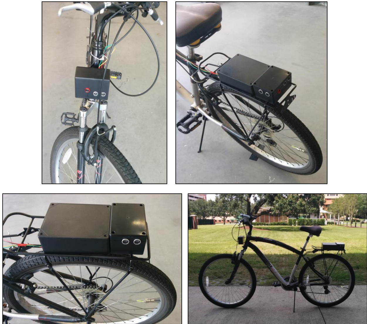
Figure 4-8 Front module and rear module of BDAS installed on bicycle.
