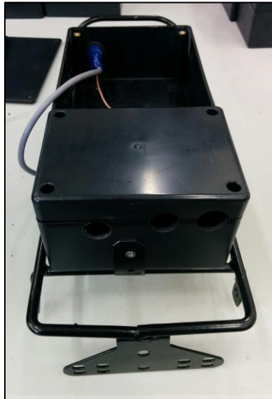
Figure 4-1 Rear enclosure with holes for camera and sensors, on a bicycle carrier rack.
