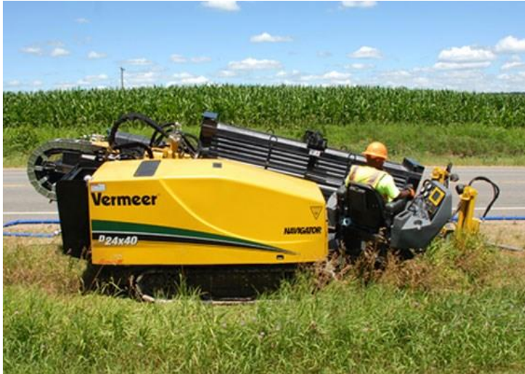
Figure 10. Horizontal Directional Drilling (HDD) Equipment.
