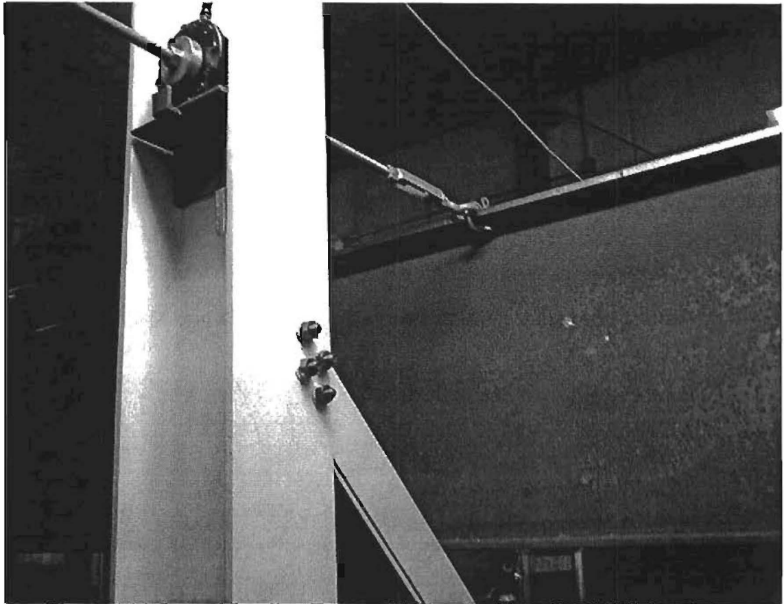
Figure 4.14 Lateral Loading Frame with Turnbuckle to Load Cell Attachment
