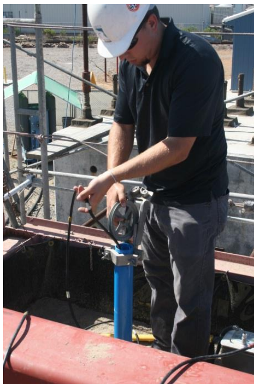
Figure 5-9: Inclinometer measurement during the test
