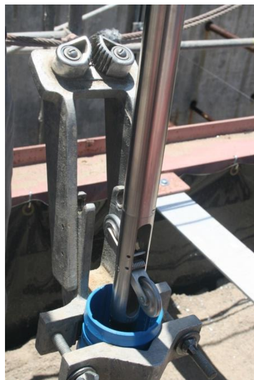
Figure 5-9: Inclinometer measurement during the test
