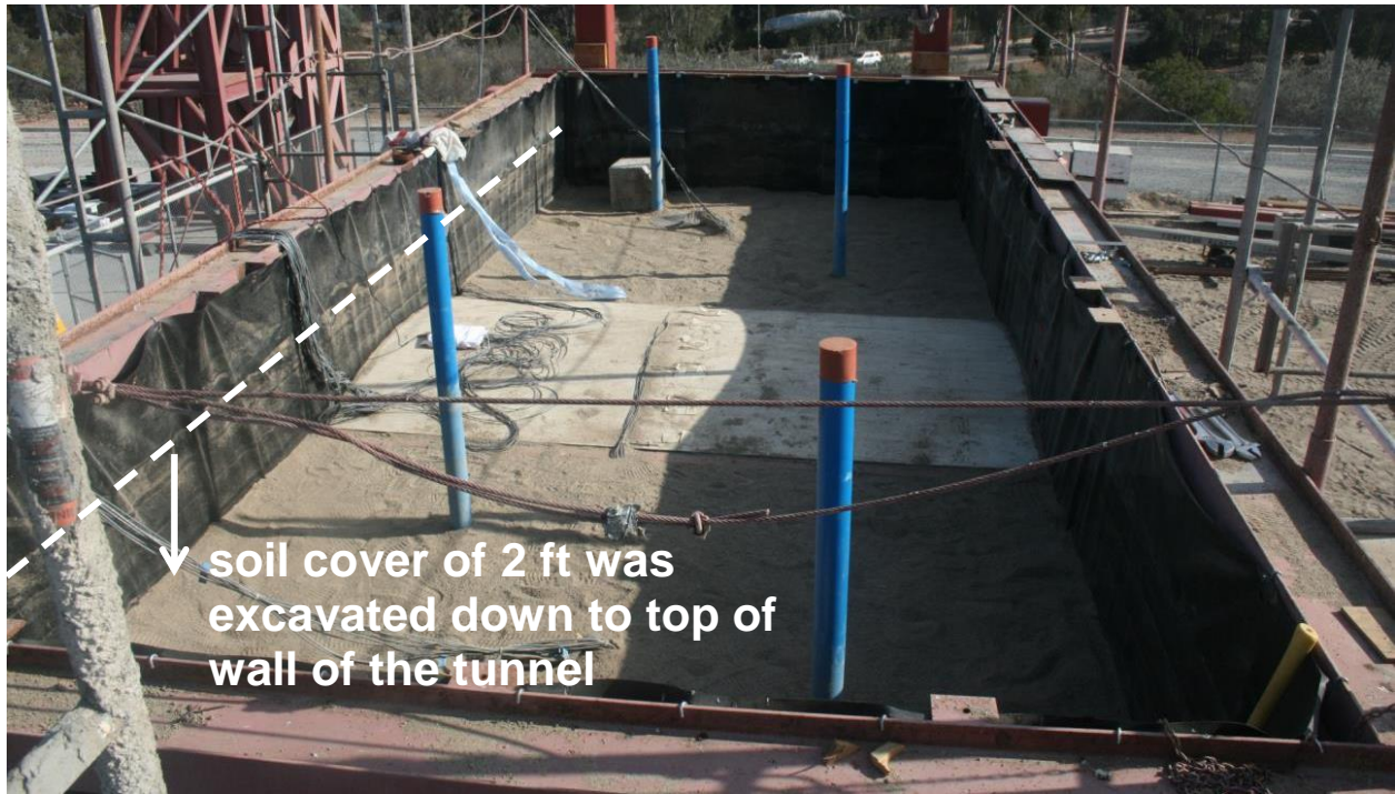
Figure 5-23: Photograph of soil surface configuration for 2 nd test
