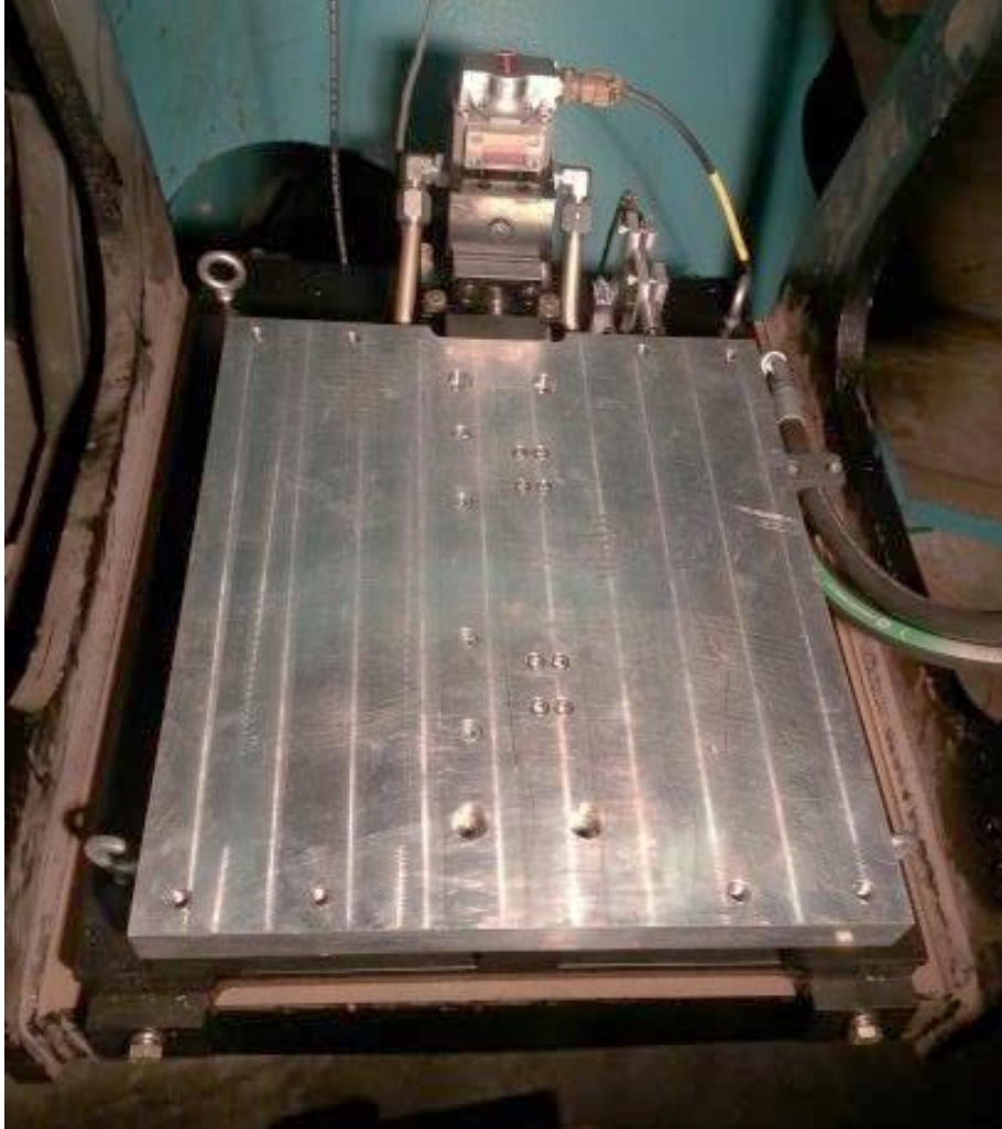
Figure 8-7: One directional servo-hydraulic centrifuge shaker
