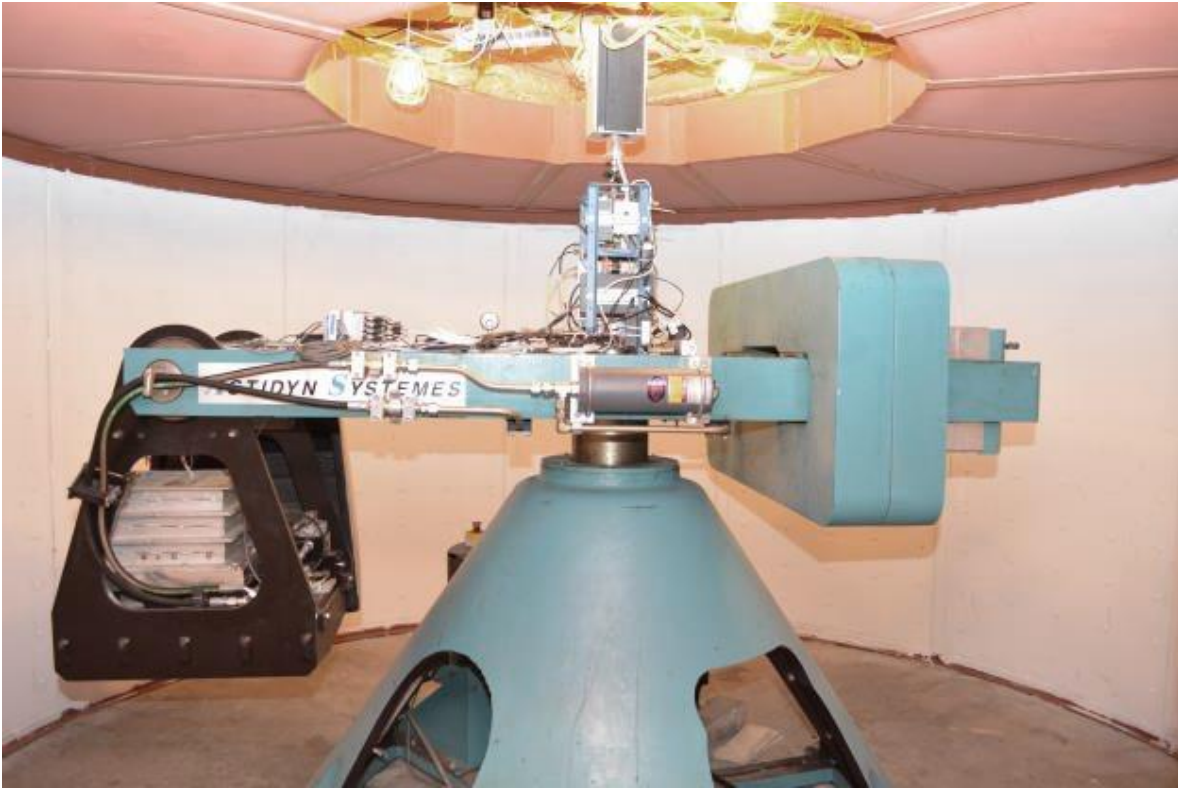
Figure 8-1: Photograph of the UCSD centrifuge
