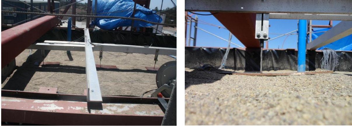
Figure 5-12: Photographs of linear potentiometers on soil surface
