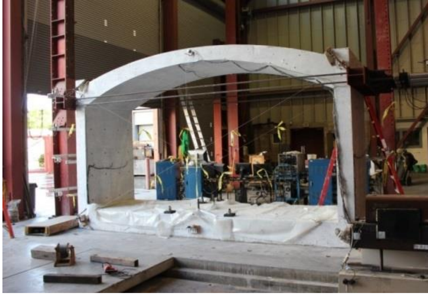
Figure 4-5: Test setup for the 1/3 scale RC tunnel subjected to cyclic loadings
