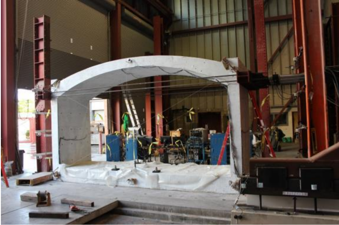
Figure C-16: Final configuration of the 1/3 reinforced concrete tunnel specimen
