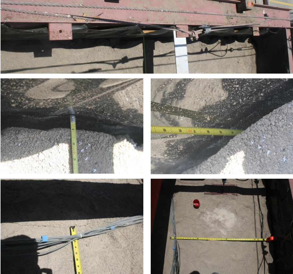
Figure 5-11: Soil separation on south side of laminar container
