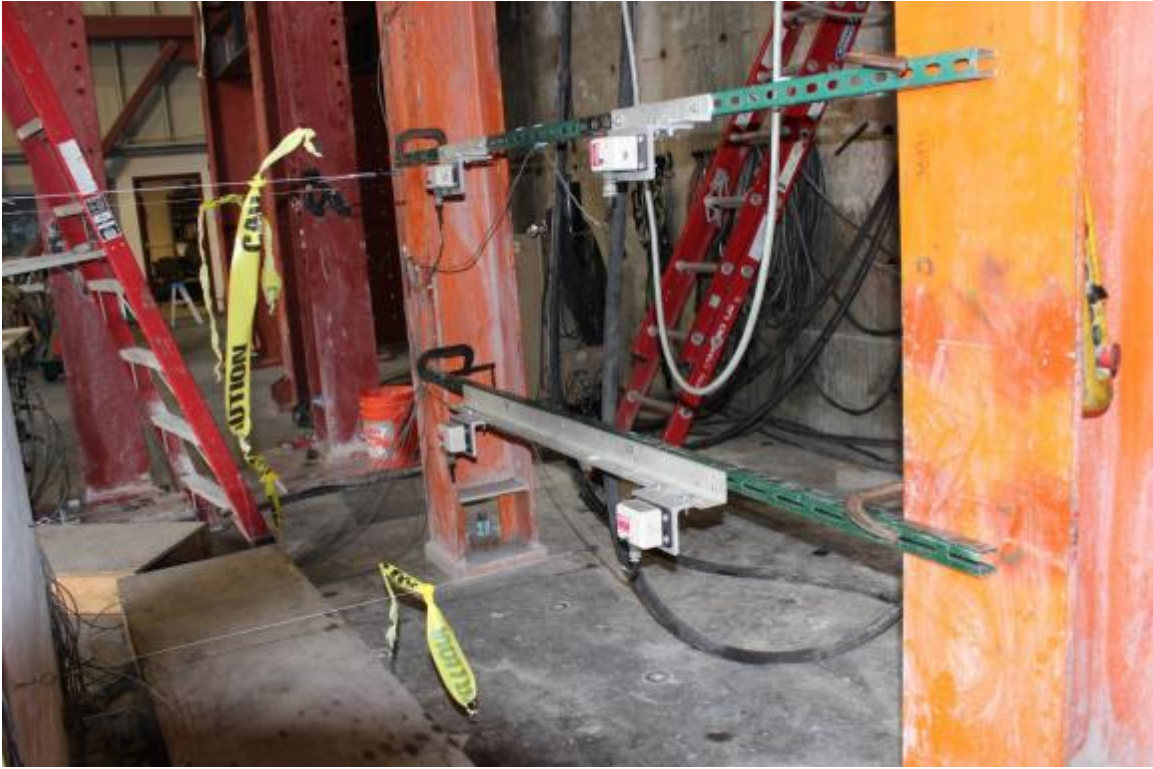
Figure C-15: Installation of the displacement transducers along the South wall
