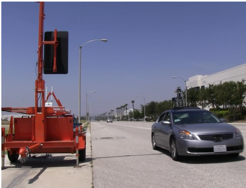
(b) Test vehicle and portable signal trailer used in the Riverside field study
