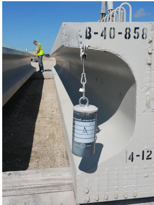
Figure 7-7 Experimental set up to measure camber
