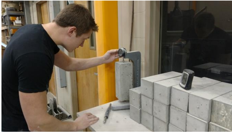
Figure 6-6 Display of shrinkage prisms sample measurement using digital length comparator
