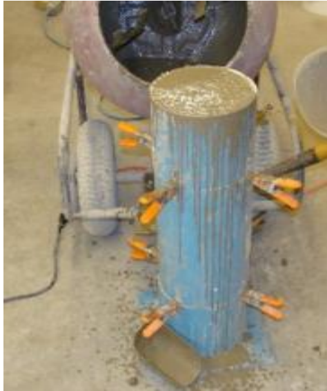
Figure 2-4 Column segregation test
