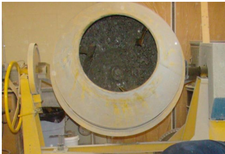
Figure 5-2 Drum used to mix SCC
