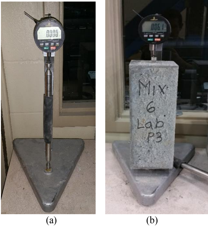
Figure 2-5 Shrinkage test setup: (a) HM-250D length comparator and (b) SCC prism specimen
