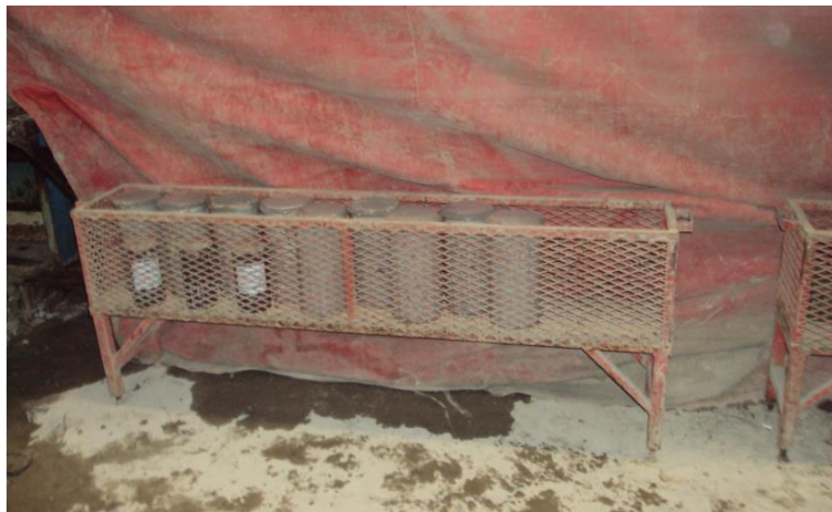
Figure 5-8 Creep samples placed adjacent to girder bed for steam curing
