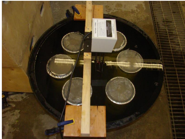
Figure 5-3 Water bath to simulate steam curing of SCC cylinders
