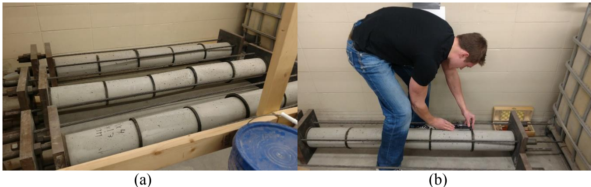
Figure 6-2 Representative pictures of creep samples: (a) all creep frames and (b) measurement taken on creep frame
