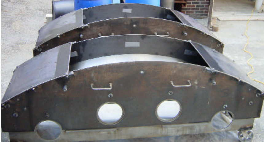
Figure 4.2.1 Molds used for casting of the pavement segments (note optional top plates at both ends)
