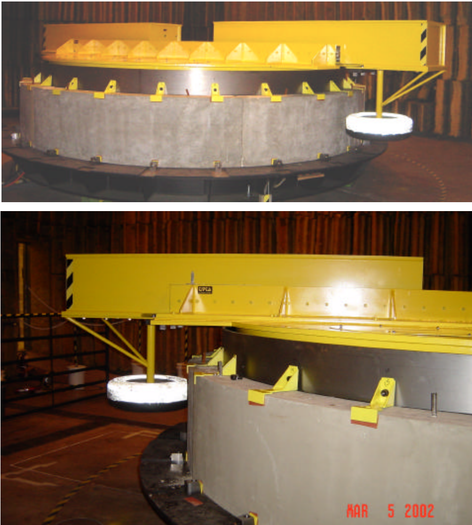
Figure 4.1.1 General view of the tire pavement test apparatus at Purdue University
