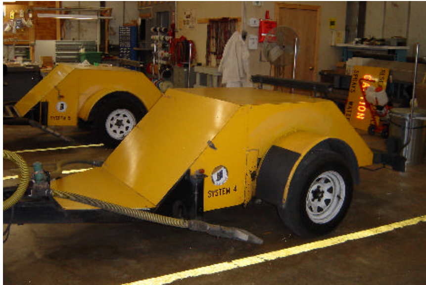
Figure 7.1.1 Skid trailer (INDOT)
