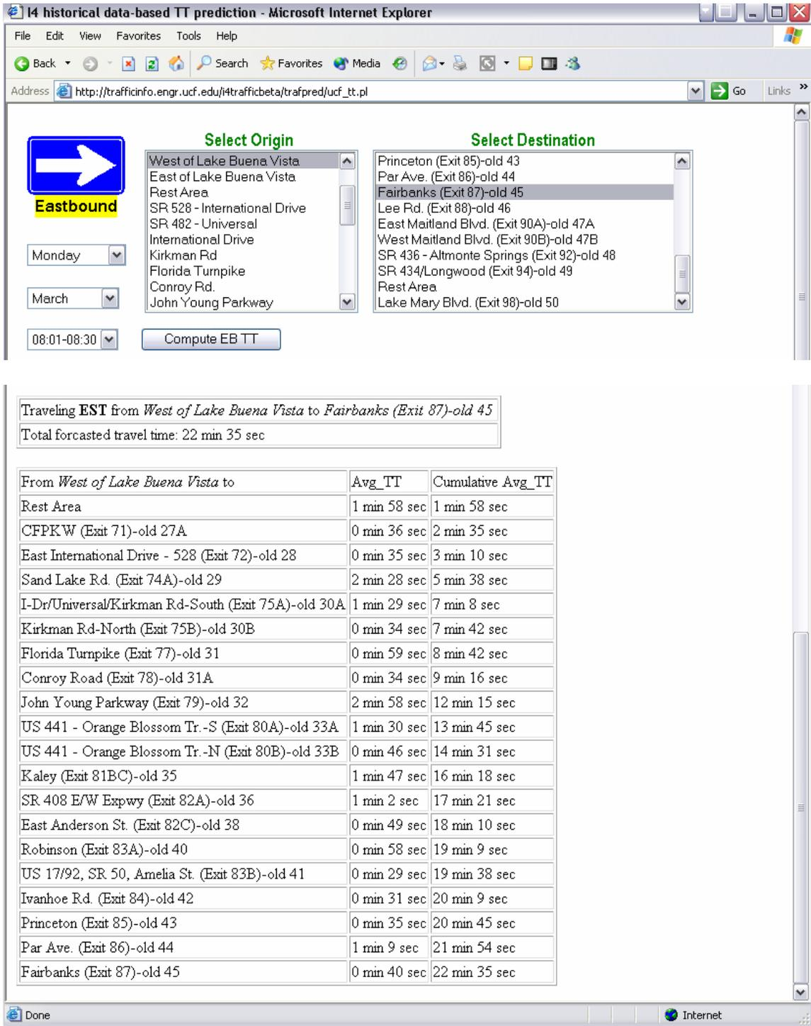
Figure 19: Snapshot of the average and cumulative long term traffic prediction in the eastbound of I-4 from West of Lake Buena Vista to Fairbanks (Exit 87)
