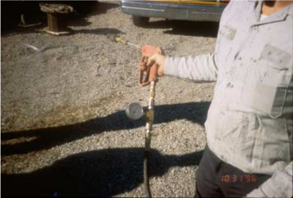
Figure 40. Line pressure gauge used to measure the washing pressure.
