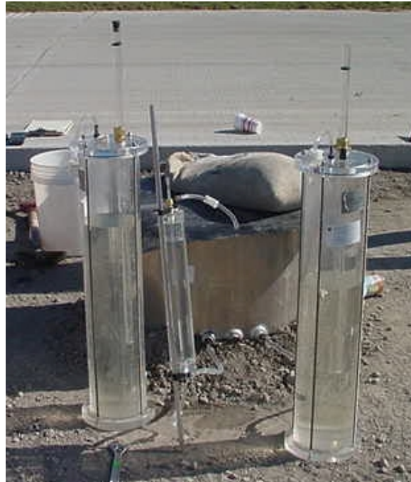
(a) Field set up of double-ring infiltrometer.
