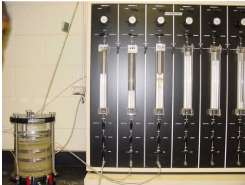
Figure 4 – Flexible-wall permeameter setup and panel board.
