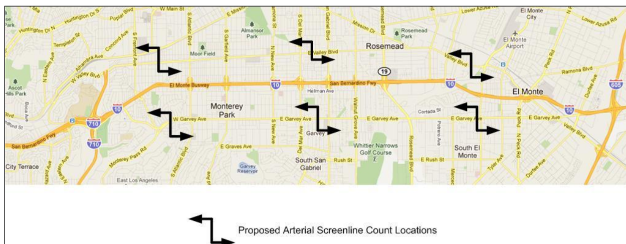
Figure 2-2. Proposed Screenline Volume Counts for Arterial Paralleling I-10
