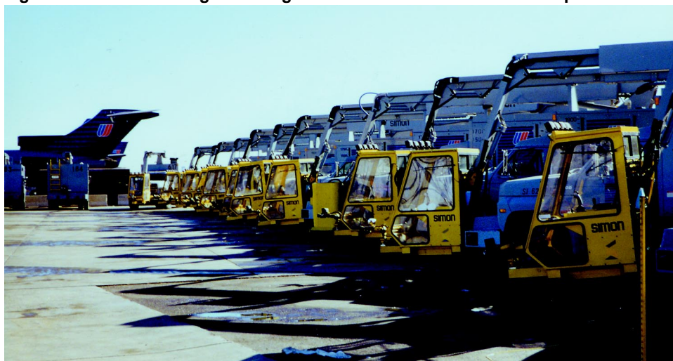
Figure 7: Aircraft Deicing/Anti-Icing Trucks at Denver International Airport
