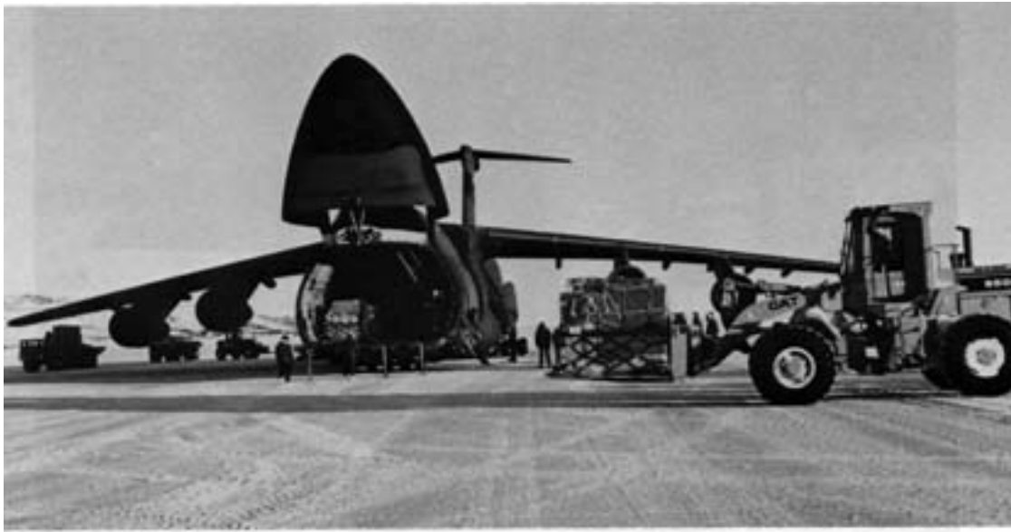
Figure 31. Lockheed C-5 Galaxy disgorging cargo through the hinged nose (19 ft wide by 13.5 ft high) at McMurdo. There is also a tail ramp (19 ft wide by 12.9 ft high), which can be used for airdrops. The maximum payload is just over 130 tons (118 tonne). The swept wings have 5.5° anhedral. After landing on ice that is almost 8 ft thick, the aircraft is unloaded, refueled and sent back north without delay. Even so, there is measurable deflection of the sea ice during unloading (several inches, or around 0.1 m). In recent years the C-5 has delivered UH-1N helicopters and a DHC-6 Twin Otter for early-season operations. (Photo by photographer's mate Oirk Meenen, USN, 3 October 1990.)
