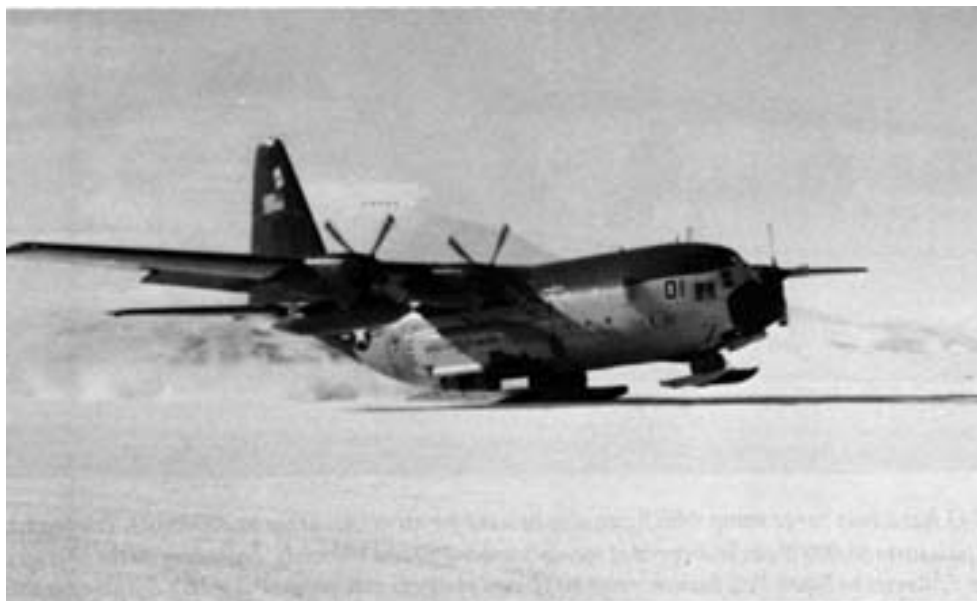
Figure 23. Lockheed LC-130R Hercules with ski-wheels (XD 01, or Buno 160741). Four of these machines, plus two of the older LC-130F, make up the USAP fleet of six ski-wheel transports. The aircraft are owned by NSF and operated by the USN (VXE-6). The 109th TAG, NYANG, has four LC-130Hs of more recent vintage. The LC-130 is used in Antarctica to supply inland stations and support field parties. (Photo by M. Mellor, 3 November 1990.)
