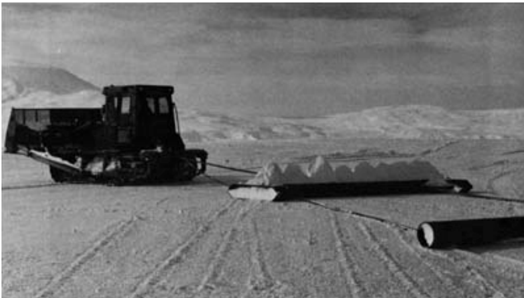
Figure 50. Simple drag for grooming skiway surfaces. The main item is a steel I-beam with improvised end skis. It is followed here by a pipe drag. (Photo by M. Mellor, November 1988.)
