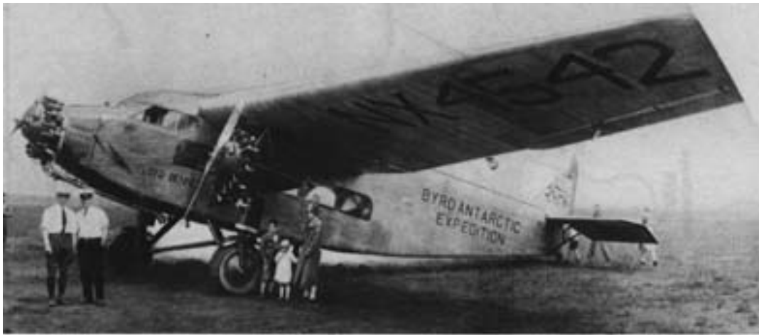
Figure 3. Ford 4T trimotor used by the Byrd Antarctic Expedition. (Smithsonian Institution photo no. 03914.)
