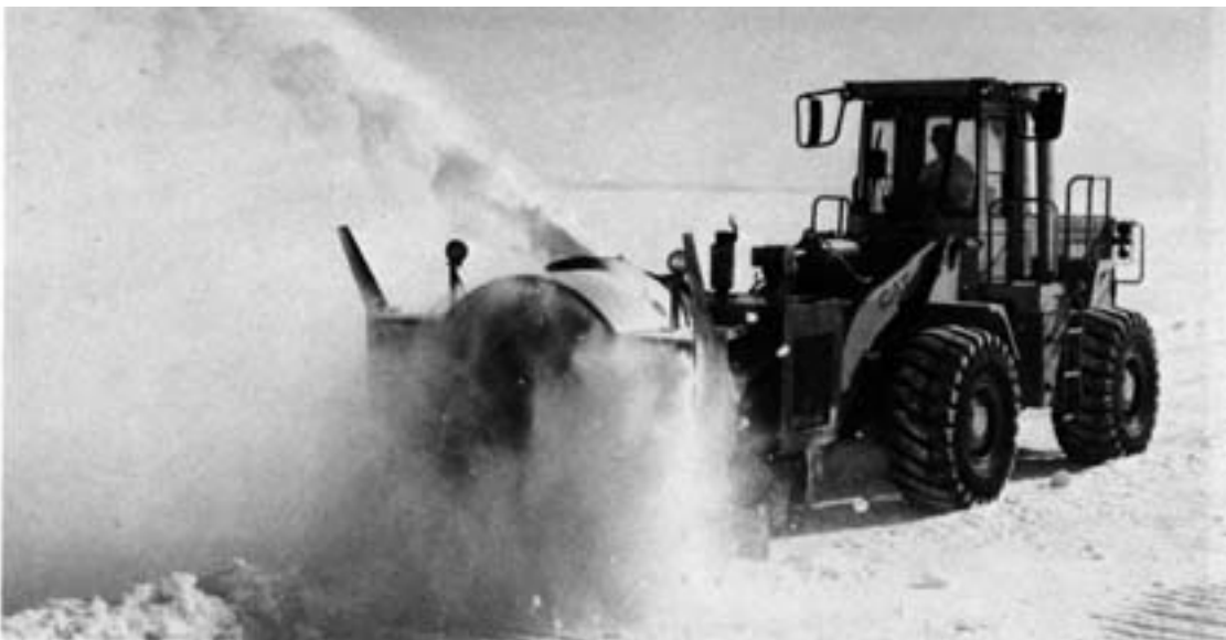
a. Single-stage, all-mechanical Blanchet with axial rotation. This unit concentrates a very heavy load on the front of the tractor when it is in the raised position.
