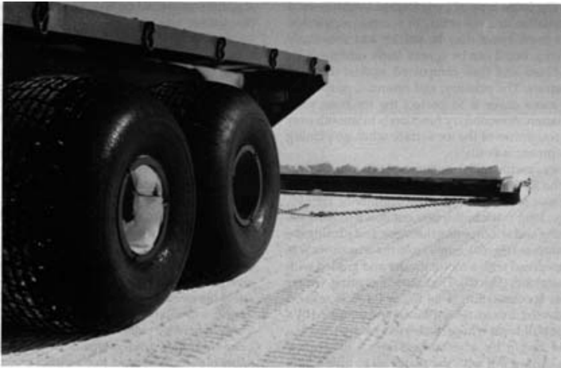
Figure 68. Foremost Delta Three towing a simple drag. Big, smooth-rib tires (as opposed to aggressive cleated tires) on a large vehicle are useful for gentle compaction. (Photo by M. Mellor, February 1990.)
