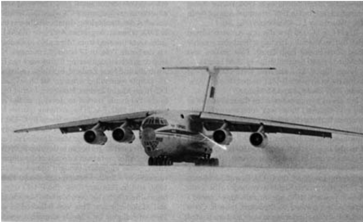
Figure 26. Ilyushin Il-76TD taking off from the compacted-snow runway at Molodezhnaya. Similar in configuration and performance to the C-141, the Il-76T (MTW 375,000 lb, four Soloviev turboprops, first flown in March 1971) is well adapted for operation from substandard airfields. Compared with the C-141, it has twice as many mainwheels, bigger tires and much lower inflation pressures. (Photo courtesy of Vladislav Piguzov, November 1990.)
