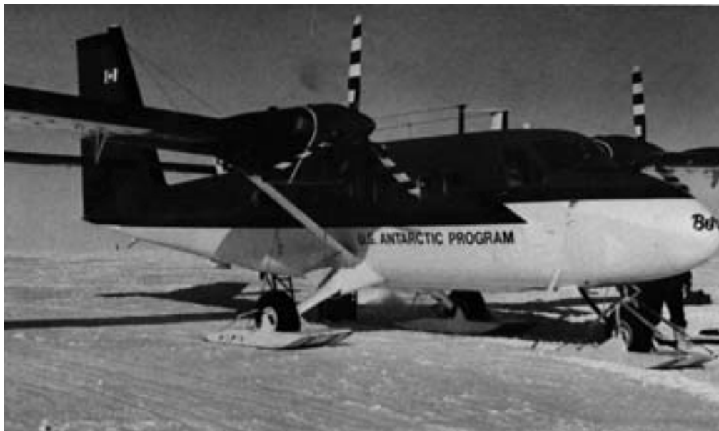
Figure 32. Ski-wheel DHC-6 Twin Otter of Kenn Borek Air at the South Pole. The Twin Otter (first flown in May 1965; MTW 12,500 lb; two 652-hp P&W turboprops) has been used in Antarctica by a number of countries for a variety of purposes, from logistics and field support to mapping photography and aerogeophysical work. Landing gear options include standard wheels, oversize “tundra tires,” hydraulic ski-wheels, fixed “penetration skis” and simple skis without wheels. In 1988-89 C-FKBG and C-FSJB (shown) operated from South Pole Station for reconnaissance, test landings and surveys at blue-ice sites in the Transantarctic Mountains. (Photo by M. Mellor, 22 January 1989.)
