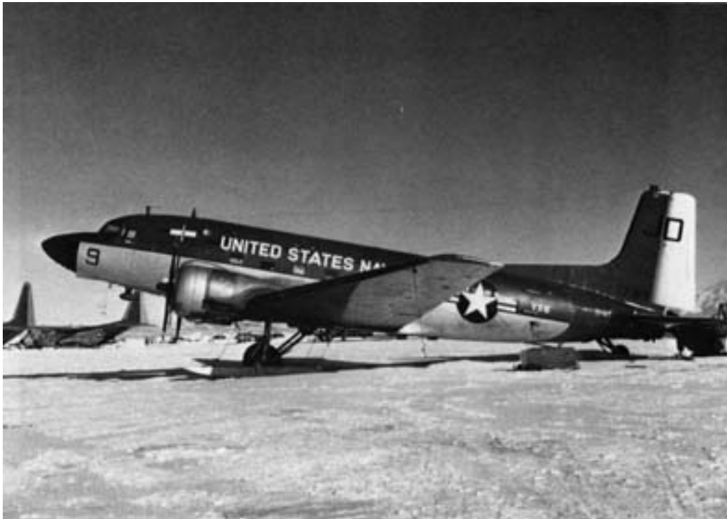
Figure 10. USN ski-wheel Douglas R4D-8 at McMurdo. A derivative of the original DC-3 (C-47) (first flown in December 1935), the R4D-8, or C-117D (MTW 31,000 lb, two 1500-hp Wright Cyclones), was the military version of the 1949 Super DC-3, or DC-3S. Standard R4Ds first entered Antarctica with Operation Highjump in 1946-47 (which abandoned six of them on the ice); they first operated for the modern USAP in 1956, and one, Que Sera Sera, made the first South Pole landing on 31 October 1956. Two R4Ds crashed in late 1959, one in November 1961, two in November 1962, two in 1964-65 and three in 1965-66. One was dropped and destroyed in 1968, the year the DC-3 retired. The landing gear was a weakness in Antarctic flying, and in 1966 they were restricted to landings on prepared runways or smooth snow. The Australians took a DC-3 to Mawson in 1960, but it was destroyed later in the year by fierce winds at the Rumdoodle runway. Altogether, over 10,000 DC-3s were built in the U.S., with more made in the U.S.S.R. as the Lisunov Li-2. (Photo by M. Mellor, October 1961.)
