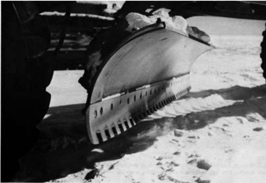
b. The blade is tilted forward to give at least 12° of relief angle beneath the tooth (even though this reduces the rake angle of the leading edge). With the blade angled to plow chips to one side, the cutting action is oblique rather than orthogonal; this reduces the kerf width and the kerf spacing. With the tooth geometry shown in these photos, there is a stub of uncut rib between the kerfs at full blade penetration. (Photos by M. Mellor, 4 February 1991.)
