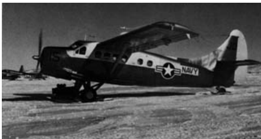
Figure 18. USN ski-wheel DHC-3 Otter (U-1A) at McMurdo. The STOL Otter was an all-tin replacement for the Noorduyn (CCF) Norseman (C-46A), a Canadian bush-flying classic. The Otter (first flown in December 1951, MTW 8000 lb, 600-hp P&W radial) was used in quantity by the USAP. For 1955-56, VX-6 (no "E" in those days) had four Otters, three of which were destroyed. For 1956-57 there were 10 Otters, and only one was lost (to wind at Little America). Two were lost in 1958-59, one in a low departure turn (or possibly stall) at Marble Point. Their role in the USAP was gradually taken over by helicopters, and they were retired from the USAP in 1966. (Photo by M. Mellor, October 1961.)
