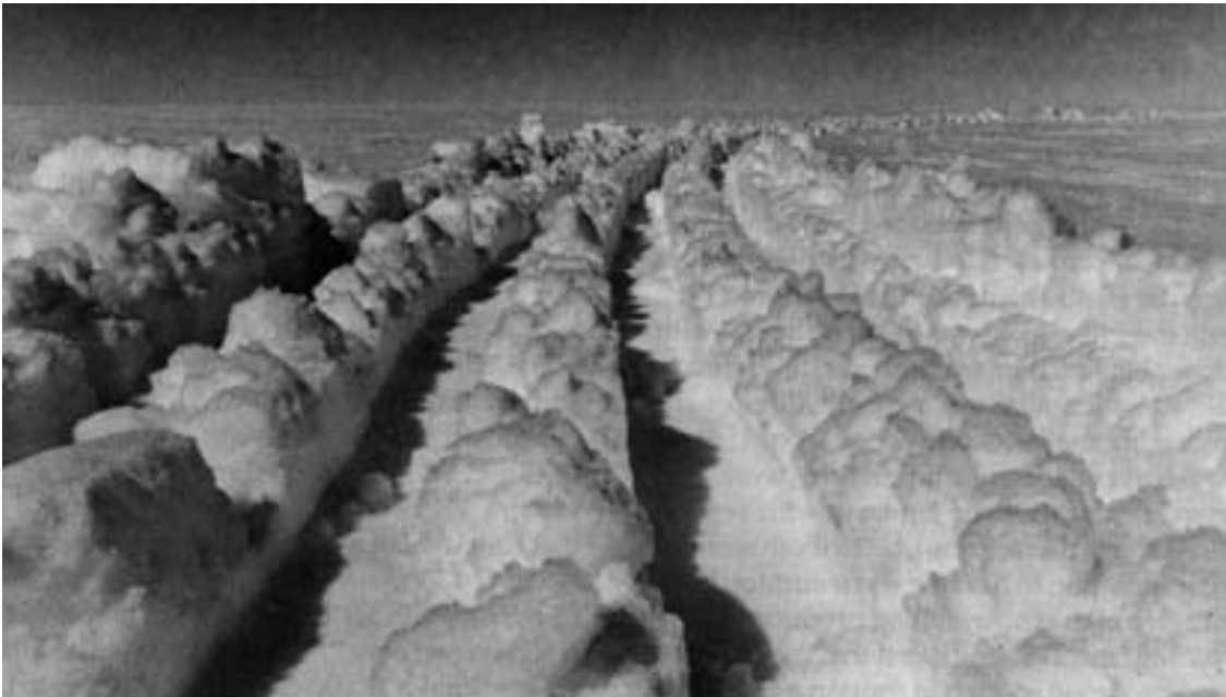
Figure 59. Deep ruts made by a heavily ballasted wheel roller after a first pass through moist snow at the 1990 Casey runway site. (Photo by Bob Sheers, Australian Antarctic Division, January 1990.)
