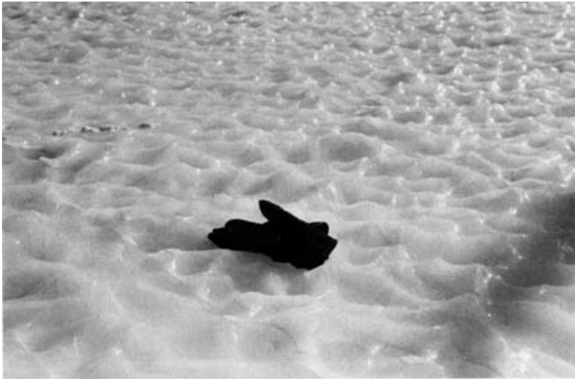
b. Scale of the cupped surface, which provides good braking and directional control. The ice evaporates at a rate of 4 in./yr (10 cm/yr).
