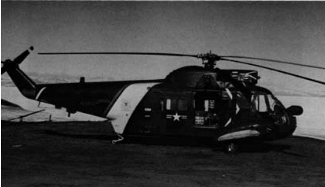
c. Sikorsky S-62 (HH-52A) helicopter, which operated from U.S. Coast Guard icebreakers in Antarctica. (Photo by M. Mellor, January 1989.)
