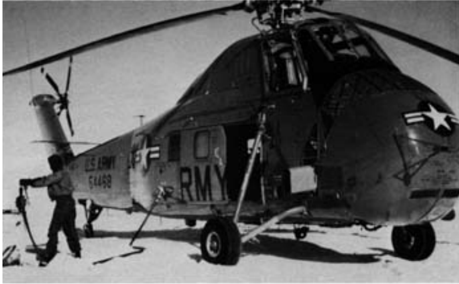
a. Piston-engine Sikorsky S-58, or H-34. Replacement of piston-engine helicopters with turbine machines greatly improved operational capabilities, e.g. in lifting field parties to high-altitude sites. Westland built a turbine version of the S-58 in the United Kingdom as the Wessex, and Sikorsky developed a turbine version as the S-58T.
