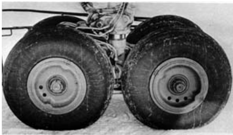
Figure 41. Wheels of the Ilyushin Il-18D. The eight 3-ft-diameter main wheels (930 × 305 mm) carry about the same gross weight as the four larger main wheels of the C-130. The standard inflation pressure is 114 lbf/in. 2 (85 lbf/in. 2 in the 700- × 250-mm nosewheels). In principle, side-by-side wheels are preferable to wheels in tandem on a snow runway, since multiple passes of a wheel over soil or snow tend to cause progressive damage and rutting. (Photo by photographer's mate Craig Peterson, USN, November 1990.)
