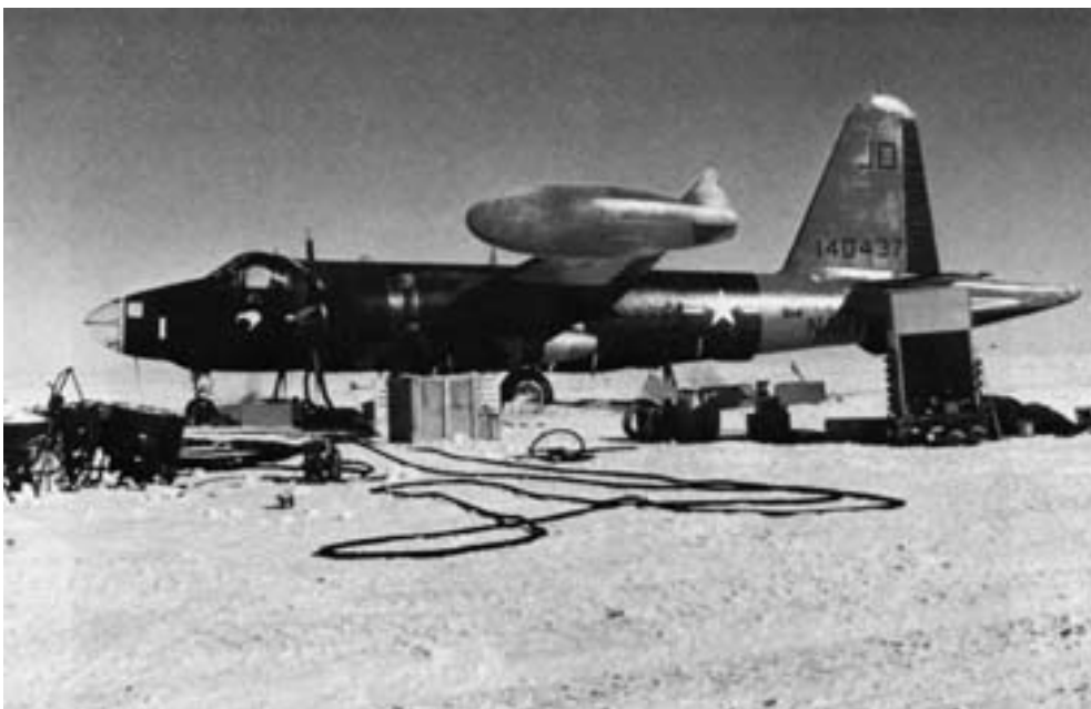
Figure 14. USN ski-wheel Lockheed P2V-7 Neptune. Introduced to Antarctica in 1956, the P2V long-range patrol bomber was used for aerial mapping photography and geophysical research. Derived from the original P2 (first flown in 1945), this Navy version eventually had two 3500-hp Wright piston engines and two 3800-lbf Westinghouse J34 turbojets, with an MTW of 80,000 lb. Two crashed in Antarctica (McMurdo, October 1956, and Wilkes, November 1961), and two assigned to Antarctic service crashed outside (one in Venezuela in February 1956 and one in California in August 1958). (Photo by M. Mellor, October 1961.)
