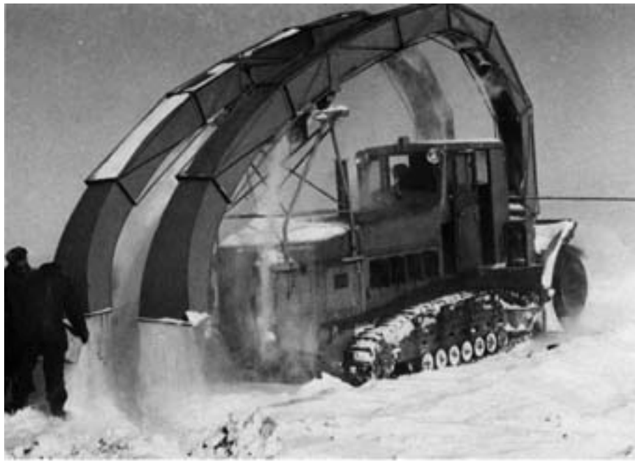
a. Peter snow miller adapted for runway processing on the Greenland Ice Cap. With the rotor running at high speed and the machine traveling slowly, the snow is milled to fine grain size. The grains deposit with relatively high initial density, and intergranular bonds form by vapor diffusion as very fine particles and sharp corners evaporate. (USA SIPRE photo.)
