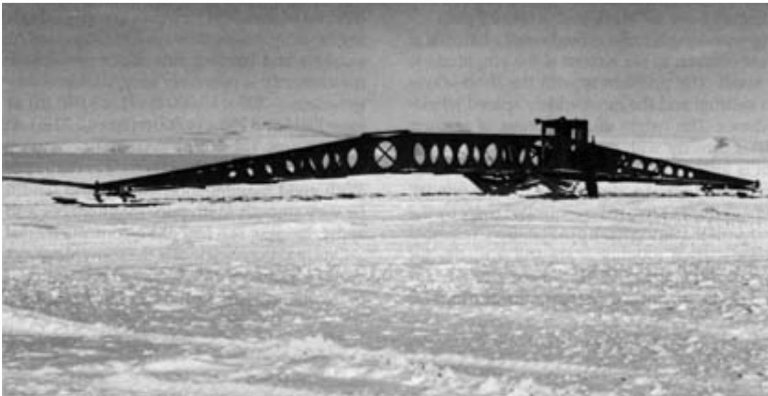
c. Eighty-ft (24-m) snowplane for subduing long-wave bumps. The long “wheelbase” gives inherent stability for fine leveling. The long trusses of this machine were plagued by structural failures in the early years. Some operator skill is required to avoid “bouncing” when the speed is too high or the bite is too deep. (Photo by M. Mellor, November 1990.)
