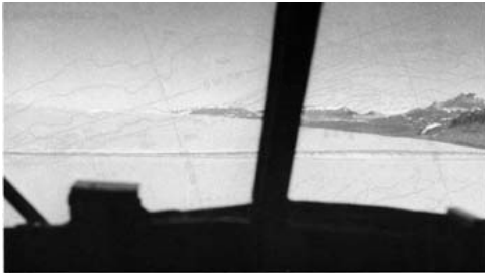
Figure 95. Low approach to Mill Glacier. For present purposes the threshold can be taken as about 3000 ft (~1000 m) beyond the Plunket Point medial moraine. The landing is normally directly into the wind, with an uphill slope averaging 1.4%. (Photo by M. Mellor, 30 November 1989.)
