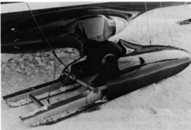
Figure 36. Dornier 228 outfitted for Antarctic service. In normal service it has retractable gear, but for Antarctic service the gear remains extended, with retractable skis over the wheels. A sleek molded fairing, reminiscent of a racing bobsled, minimizes aerodynamic drag. (Photo by photographer's mate Craig Peterson, USN, December 1990.)
