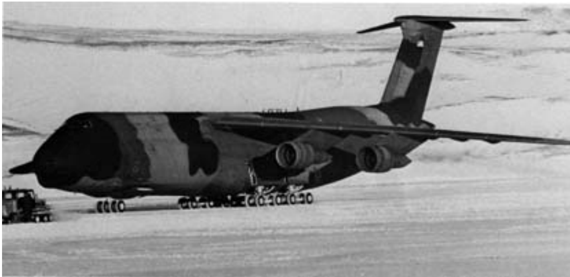
Figure 30. Lockheed C-5 Galaxy of MAC on the sea ice at McMurdo. At an MTW of 840,000 lb, very thick ice (> 8 ft) is needed if the aeroplane parks for any length of time. The aircraft currently operates to McMurdo only in early October, when the sea ice is near its maximum thickness and is still very cold. The C-5 (first flown in June 1968) got off to a shaky start but came into its own after 1981, when new wings were retrofitted to the original C-5A; deliveries of the C-5B started in 1986. The MLG has two triangular units, each with six wheels, on each side, for a total of 24 wheels. The nose unit has four wheels. The C-5 is driven by four GE turbofans, each developing 43,000 lbf of thrust. The cruising speed is 450 knots, making this the fastest aeroplane in current Antarctic service, as well as the largest. (Photo by photographer’s mate Oirk Meenen, USN, 3 October 1990.)
