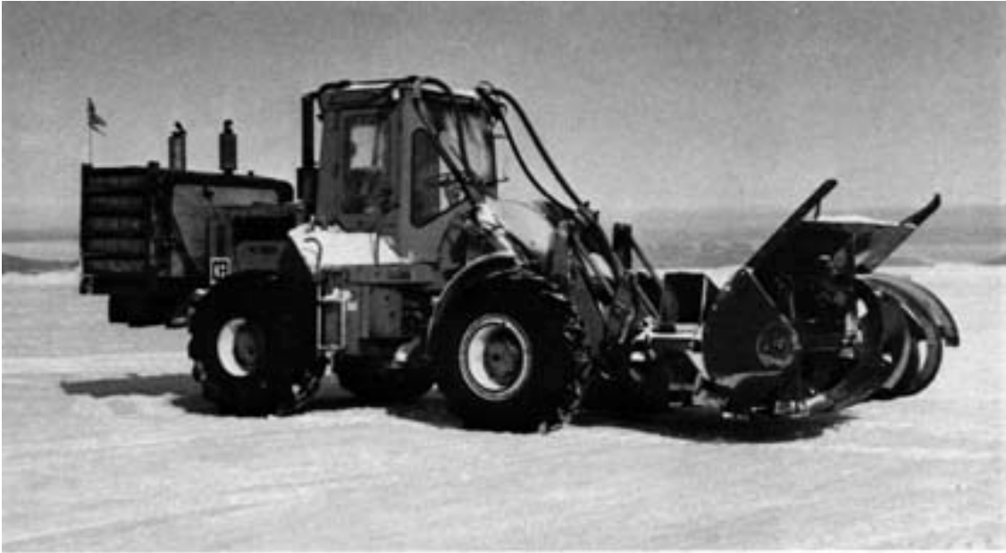
b. Two-stage, hydraulic-drive Snowblast with transverse-rotation auger and axial-rotation impeller. This unit distributes the load, but there is an unavoidable power loss in the hydraulic drive.
