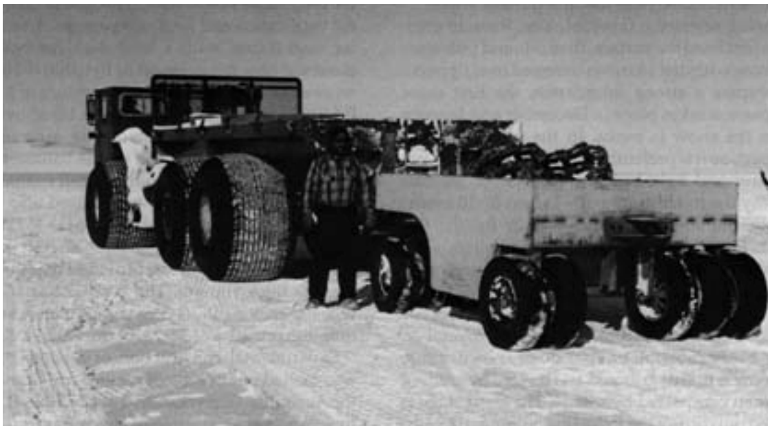
b. Small U.S. compaction roller (a 13-wheel roller with one pair of wheels missing in this photo). Both roller and wheels are believed to be too small for efficient compaction of runway pavements. The wheels of the Delta vehicle make excellent rollers for the snow surface, but they are too lightly loaded to achieve deep compaction. (Photo by M. Mellor, November 1990.)
