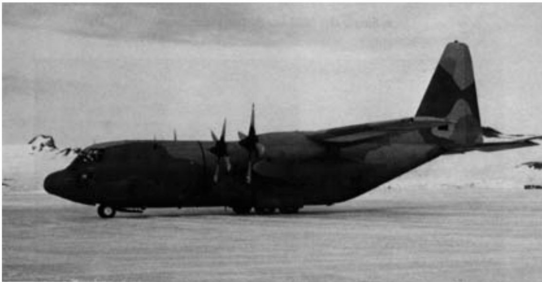
Figure 21. Lockheed C-130 Hercules on the sea ice at McMurdo. The standard C-130, on wheels only, first flew to Antarctica in late 1959. Currently a Hercules of 40 Squadron, RNZAF (illustrated), maintains a passenger and freight service between Christchurch and McMurdo from October to early December. There are also occasional Hercules flights to McMurdo by the Italian Air Force and the RAAF (36 Squadron). In the Peninsula, flights to Marsh and Marambio are made by the USAF, FACH, FAA and the Brazilian Air Force. The C-130 Hercules (prototype first flown in August 1954, production model first flown in April 1955) has gone through many stages of development. The C-130H has four 4500-hp Allison turboprops, an MTW of 175,000 lb and a 300-knot cruising speed. Passenger amenities have remained at cattle-truck standards for over three decades. (Photo by M. Mellor, November 1990.)
