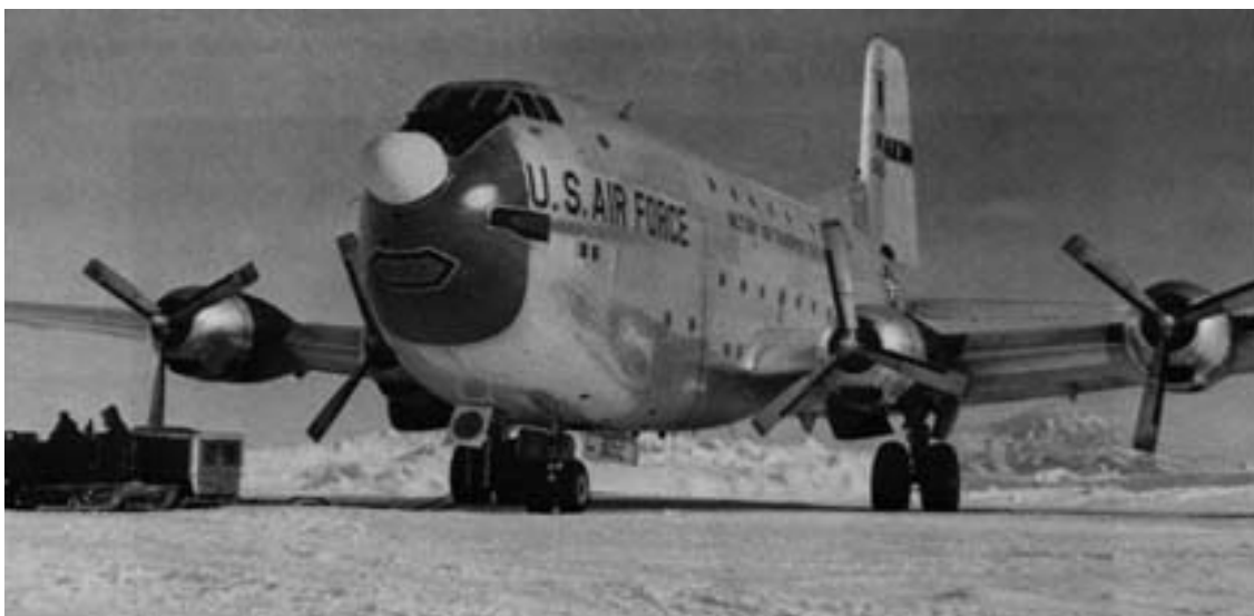
Figure 16. USAF Douglas C-124 Globemaster II on the sea ice at McMurdo. The C-124 (first flown in November 1949) had an MTW of 194,500 lb and four 3800-hp P&W (Ford) radials; 446 were built. It had nose doors with ramps and a rear hatch with an elevator, and it could accommodate double-decker loading. The C-124 began flights to Antarctica on 20 October 1956, and State of Oregon made the first South Pole cargo drop on 26 October 1956; 760 tons of materials were delivered by C-124s for construction of the original South Pole Station. The ride from Christchurch, New Zealand, to McMurdo was noisy and slow, with a 200-knot cruising speed. A 124 was badly damaged in a nosewheel landing at McMurdo in October 1956, and another landed short and was destroyed in November 1956. One crashed near Hallett in October 1958. The 124 was retired from Antarctic service about 1965. (Photo by M. Mellor, November 1962.)
