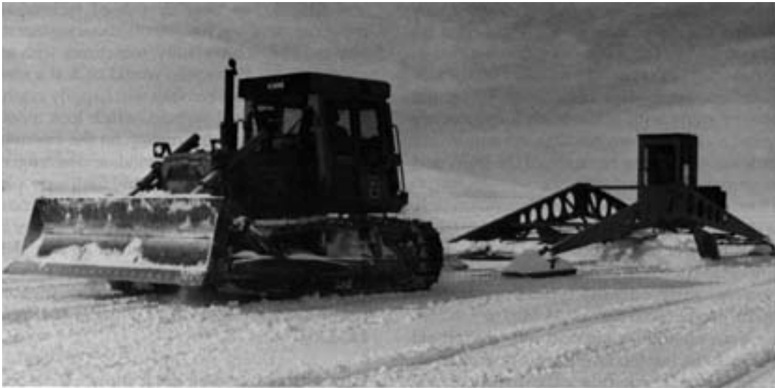
b. Forty-ft (12-m) snowplane working at Williams Field. The machines are operated manually, like simple graders, with on-board hydraulic power to actuate the blade. (Photo by M. Mellor, 1987.)
