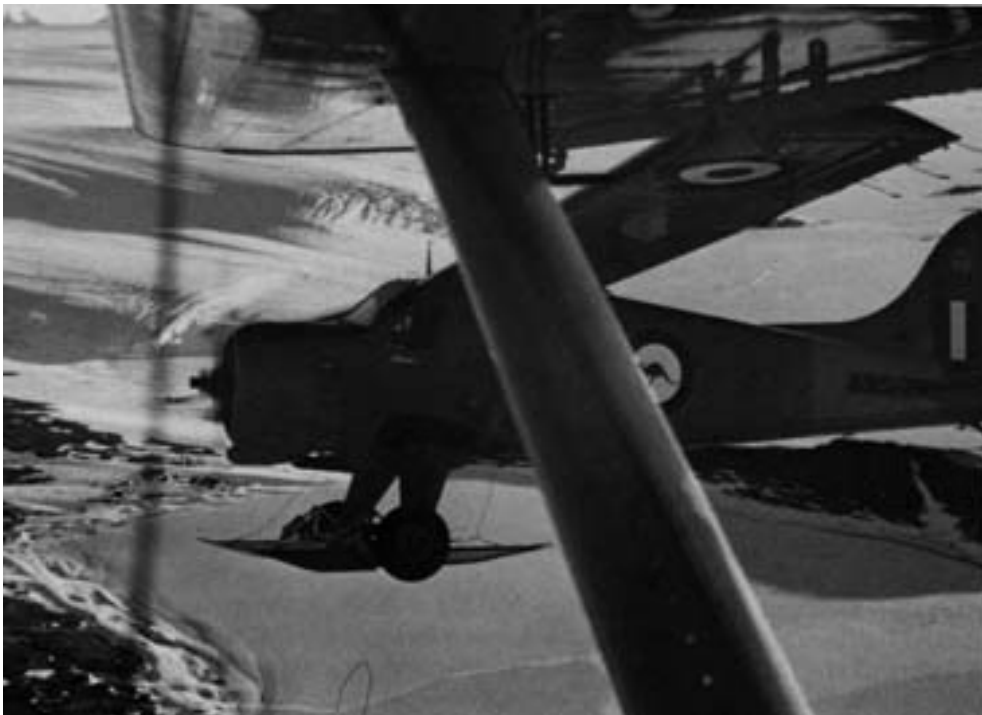
Figure 17. ANARE ski-wheel DHC-2 Beaver over Mawson (A95-202 from A95-201). The standard Beaver had an MTW of 5100 lb (2300 kg), but these operated at 5600 lb (2540 kg). The engine was a 450-hp P&W radial. A95-201 was at Mawson from 1956 to 1958; it returned in January 1959 and was destroyed by a 96-knot blizzard (along with A95-203) at the Gwamm runway in December 1959 (after being ground-flown for two hours). A95-202 stayed at Mawson from 1956 to 1959; it returned in February 1960 (via Davis) and was destroyed by a blizzard at the Rumdoodle runway in December 1960. (Photo by M. Mellor, September 1957.)
