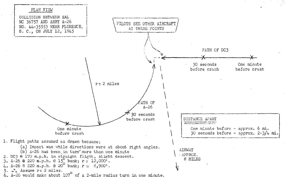
NOTE: This diagram is based on collision during flight at right angles. There is some evidence to indicate that the angle of contact was slightly more than 90°. However, if this were the case the above figures would not be changed substantially.
