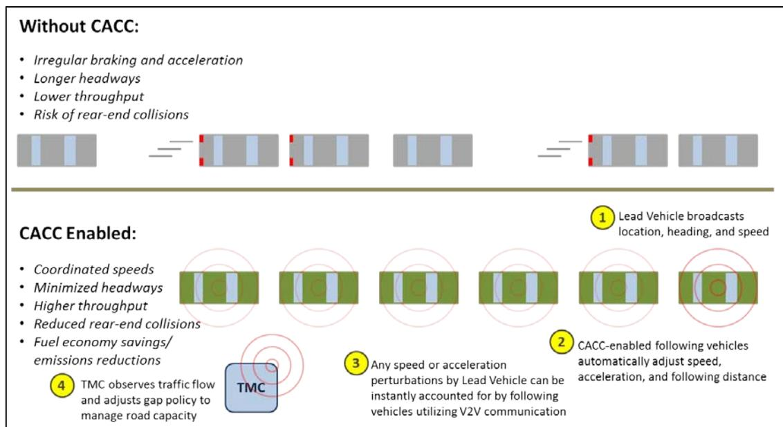
**Figure 5-3. Stylized Depiction of Connected Vehicle-Enabled CACC**
