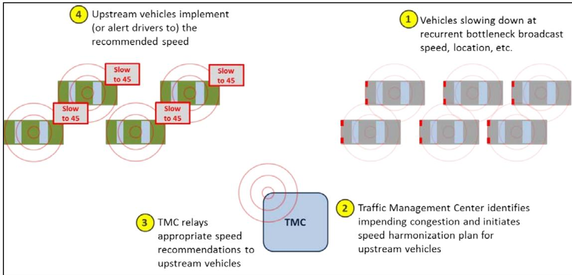
**Figure 5-1. Stylized Depiction of a Connected Vehicle-Enabled SPD-HARM Application**
