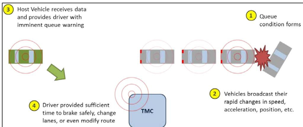
**Figure 5-2. Stylized Depiction of a Connected Vehicle-Enabled Q-WARN Application**
