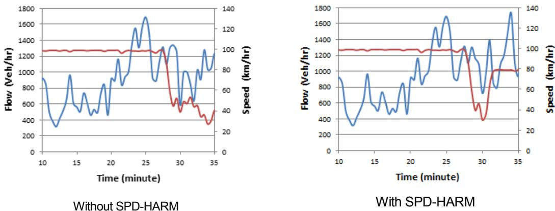
**Figure 8-1. Effect of Speed Harmonization on Flow Breakdown Elimination.**
