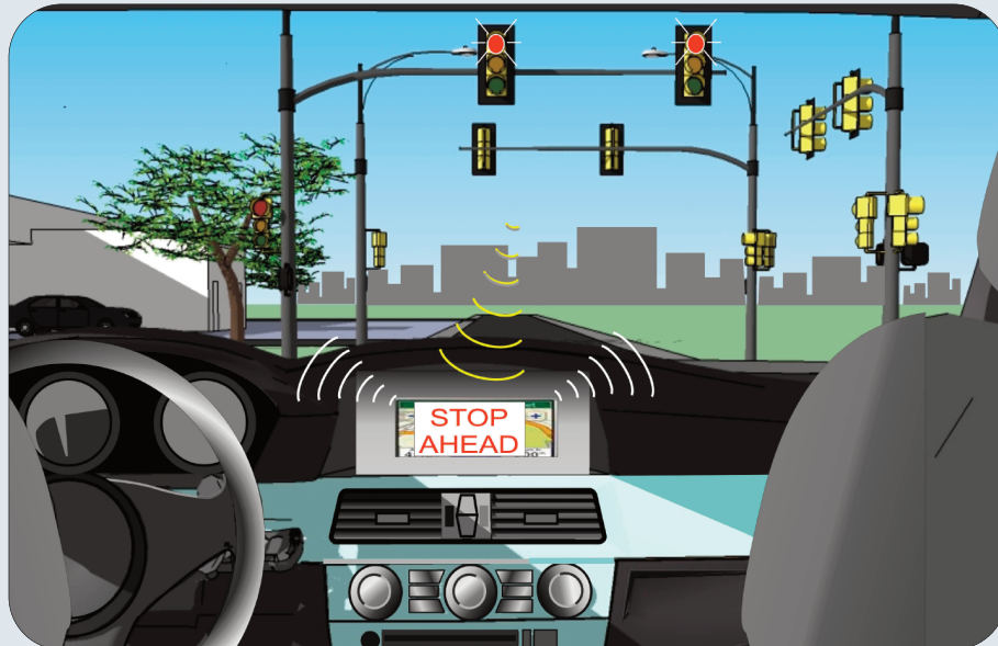
Figure 6: Signal Phase and Timing (SPaT) broadcast message.
