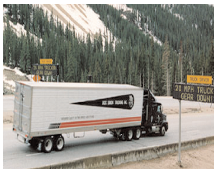
Colorado Downhill Truck Speed Advisory System integrates weigh-in motion (WIM) and dynamic message signs (DMS). 19
