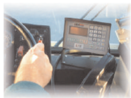
Utah’s TCP system issues a “hold” message on a transit vehicle’s MDT. 111
