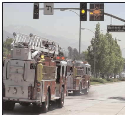
Fire trucks safely traverse an intersection equipped with emergency vehicle preemption and visual warning system. 87
