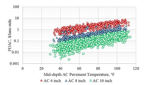
Figure B.9. Fatigue cracking based PDAC output from Monte-Carlo simulations for Mercury weather station.
