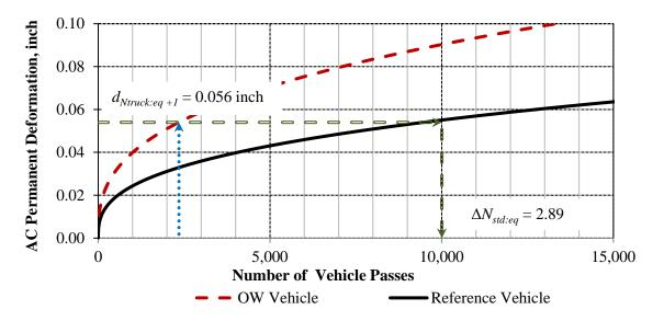
Figure 2.13. Additional number of reference vehicle passes to reach *d*<sub>truck:eq+1</sub>.
