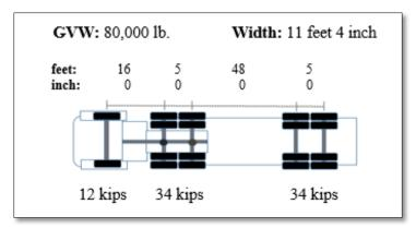
Figure 2.7. Reference vehicle configuration.
