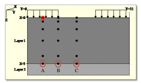
Figure 4.1. Schematic of 3D-Move analysis of a tandem axle group at six different pavement depths.
