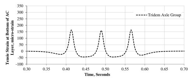
Figure 2.3. Graph. Tensile strain response history at the bottom of AC layer for axle group B (tridem axle).
