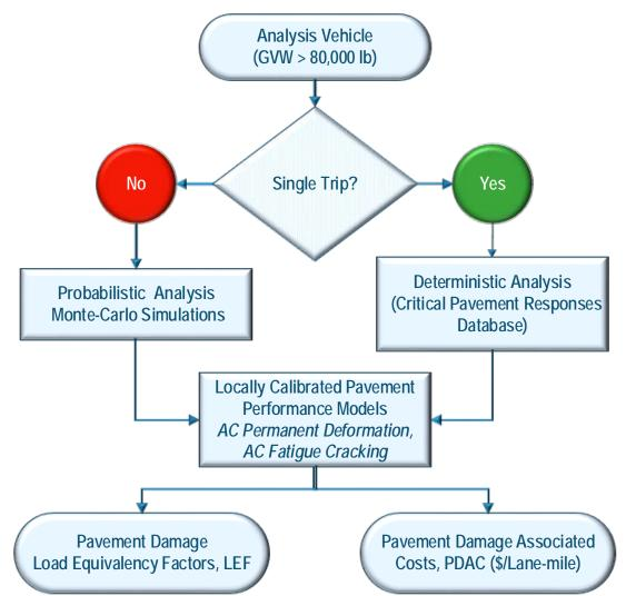
Figure 5.1. Overall methodology for determining pavement damage and PDAC.
