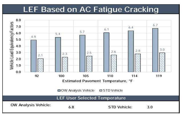
Figure 6.8. AC fatigue cracking-based LEFs output result for single trip scenario.
