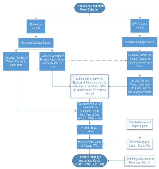
Figure 2.5. Flowchart of overall approach for the estimation of pavement damage and allocated cost.
