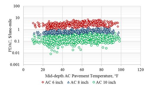
Figure B.3. Fatigue cracking based PDAC output from Monte-Carlo simulations for Ely weather station.
