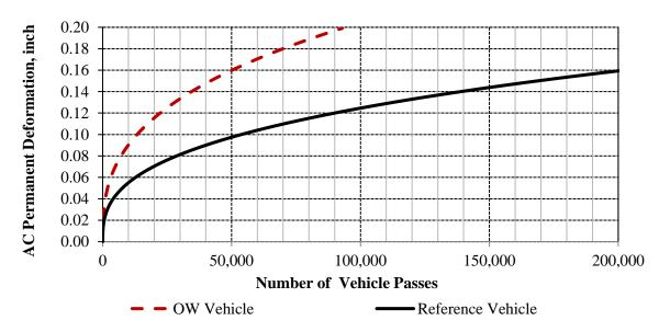
Figure 2.8. AC permanent deformation damage curves under OW and reference vehicles.
