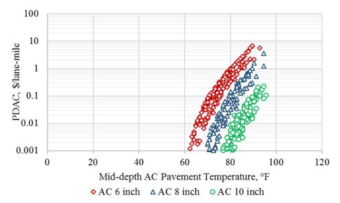
Figure B.14. AC permanent deformation based PDAC output from Monte-Carlo simulations for South Tahoe weather station.
