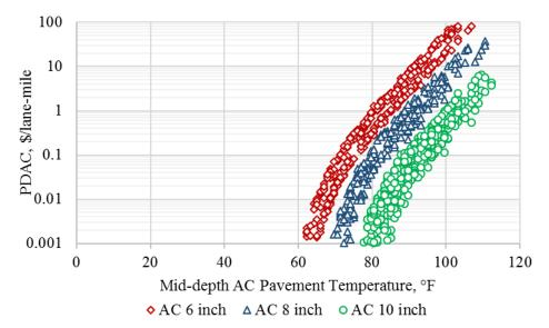
Figure B.12. AC permanent deformation based PDAC output from Monte-Carlo simulations for Reno weather station.
