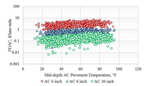
Figure B.13. Fatigue cracking based PDAC output from Monte-Carlo simulations for South Tahoe weather station.
