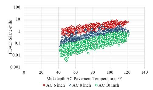
Figure B.7. Fatigue cracking based PDAC output from Monte-Carlo simulations for Las Vegas weather station.
