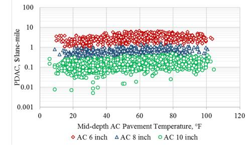
Figure B.1. Fatigue cracking based PDAC output from Monte-Carlo simulations for Elko weather station.
