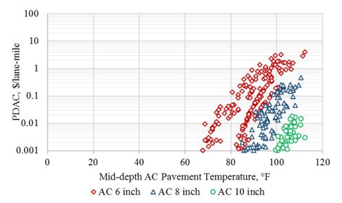
Figure B.16. AC permanent deformation based PDAC output from Monte-Carlo simulations for Tonopah weather station.
