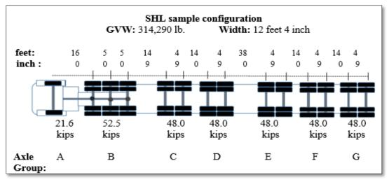
Figure 2.1. Example for an OW vehicle configuration.
