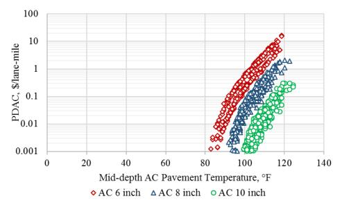
Figure B.8. AC permanent deformation based PDAC output from Monte-Carlo simulations for Las Vegas weather station.
