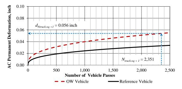
Figure 2.12. AC permanent deformation after *N*<sub>truck: eq+1</sub>.
