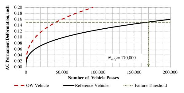
Figure 2.9. Number of reference vehicle passes to failure.
