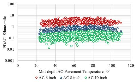
Figure 5.5. AC fatigue cracking based PDAC output from Monte-Carlo simulations for Reno weather station.
