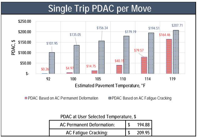
Figure 6.6. PDAC output results in US dollars for a single trip scenario.
