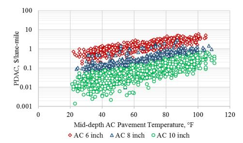
Figure B.15. Fatigue cracking based PDAC output from Monte-Carlo simulations for Tonopah weather station.
