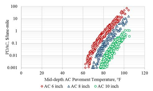
Figure B.6. AC permanent deformation based PDAC output from Monte-Carlo simulations for Lovelock weather station.
