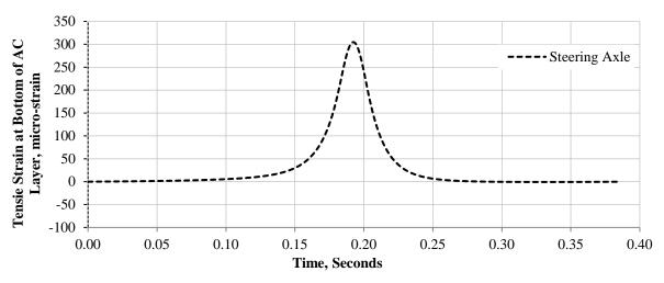
Figure 2.2. Tensile strain response history at the bottom of AC layer for axle group A (single axle).
