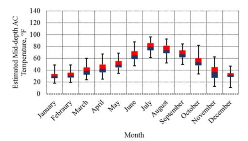
Figure 3.16. Estimated mid-depth AC temperature for South Tahoe.
