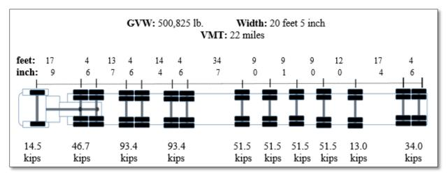
Figure 2.6. OW vehicle configuration.
