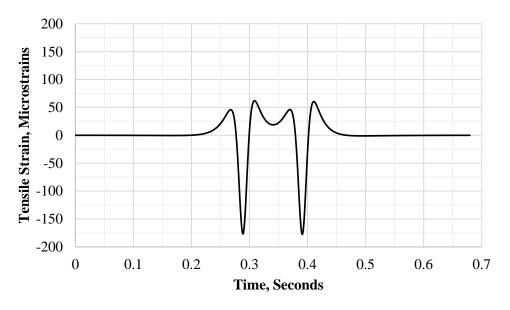
Figure 4.2. Tensile strain history at bottom of AC layer at C location (between adjacent tires).
