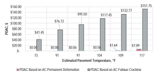
Figure 7.8. OW vehicle PDAC values in US dollars per trip for Case study II (Interstate 15 Section).
