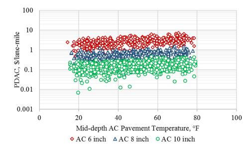
Figure B.17. Fatigue cracking based PDAC output from Monte-Carlo simulations for Winnemucca weather station.
