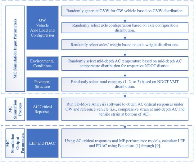
Figure 5.4. Monte-Carlo simulation flowchart presenting inputs, process, and outputs.
