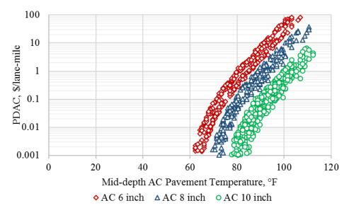
Figure 5.6. AC permanent deformation based PDAC output from Monte-Carlo simulations for Reno weather station.
