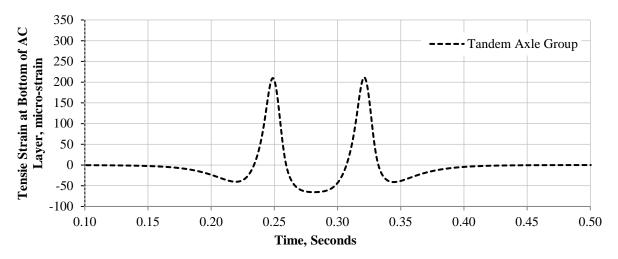
Figure 2.4. Graph. Tensile strain response history at the bottom of AC layer for axle groups C, D, E, F, and G (tandem axle).
