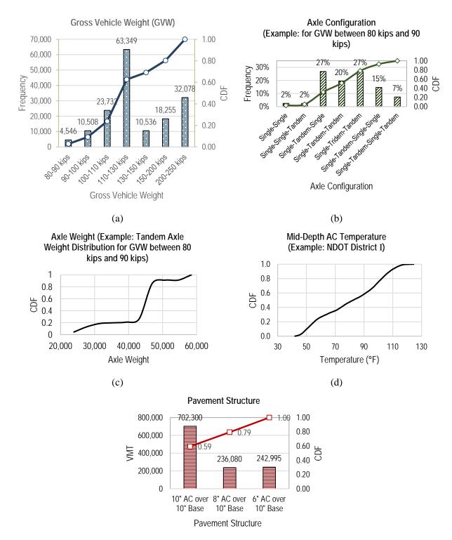
Figure 5.3. Sample input parameters for Monte-Carlo simulation: (a) gross vehicle weight (GVW), (b) axle configuration, (c) axle weight, (d) mid-depth AC temperature; and (e) pavement structure.
