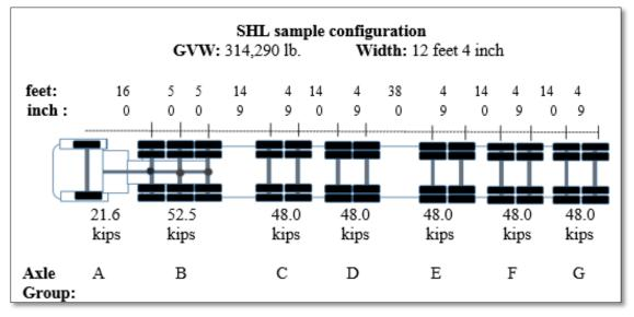
Figure 3.11. Configuration of a permitted OW vehicle.
