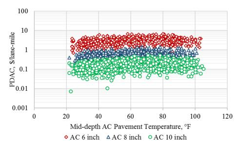
Figure B.5. Fatigue cracking based PDAC output from Monte-Carlo simulations for Lovelock weather station.
