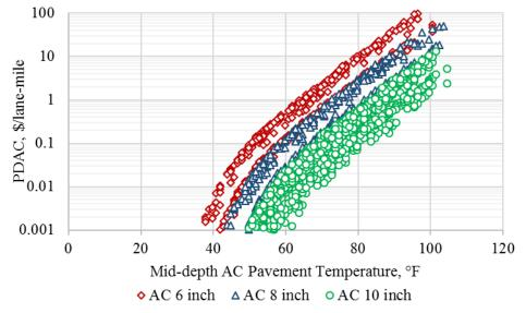
Figure B.2. AC permanent deformation based PDAC output from Monte-Carlo simulations for Elko weather station.
