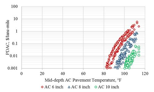
Figure B.10. AC permanent deformation based PDAC output from Monte-Carlo simulations for Mercury weather station.
