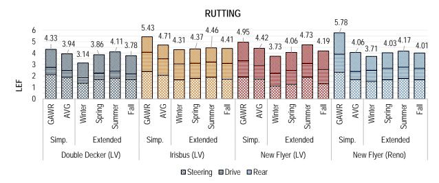
Figure 7.26. LEFs results based on AC permanent deformation.
