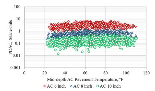
Figure B.11. Fatigue cracking based PDAC output from Monte-Carlo simulations for Reno weather station.
