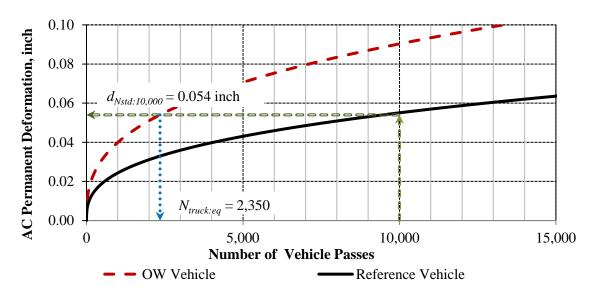
Figure 2.11. Equivalent number of OW vehicle passes after 10,000 passes of the reference vehicle.
