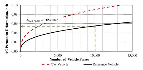
Figure 2.10. AC permanent deformation after 10,000 passes of reference vehicle.
