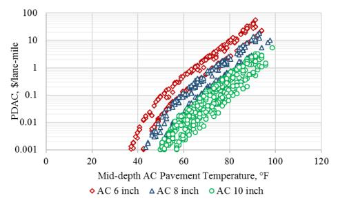
Figure B.4. AC permanent deformation based PDAC output from Monte-Carlo simulations for Ely weather station.
