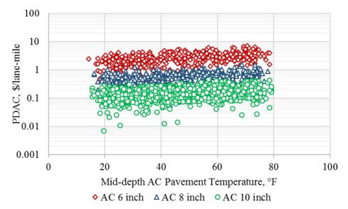
Figure B.18. AC permanent deformation based PDAC output from Monte-Carlo simulations for Winnemucca weather station.
