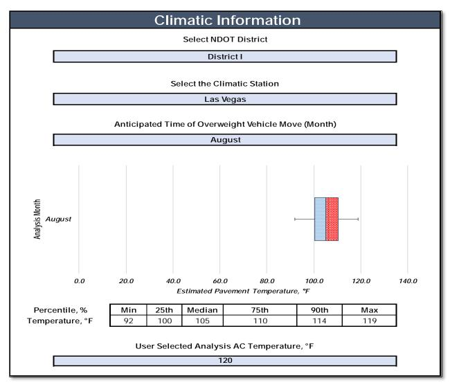
Figure 6.1. Climatic Information input panel for single-trip analysis.
