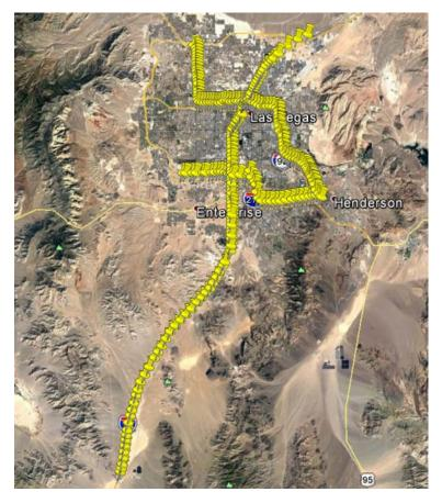
Figure 2-1. Inductive loop detector locations of received ITS data
