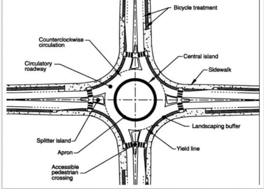
**Apron:** The mountable portion of the central island adjacent to the circulatory roadway required to accommodate the wheel tracking of large vehicles. Sometimes the apron is provided on the outside of the circulatory roadway.
