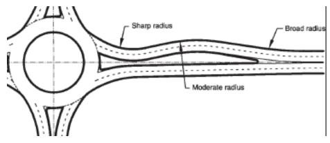
Figure 25: Successive Curves on High Speed Approaches Source: NCHRP Report 672
