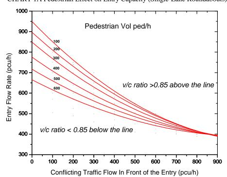
CHART 1A Pedestrian Effect on Entry Capacity (Single-Lane Roundabouts)
