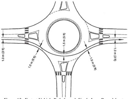
Figure 13: Fastest Vehicle Path through Single-Lane Roundabout Source: NCHRP Report 672
