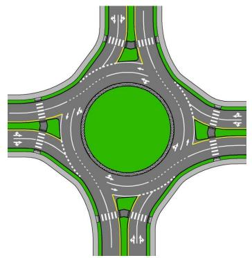
Figure 7: Lane Arrangements for Typical Double-Lane Roundabout Source: MUTCD 2009
