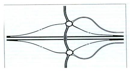
Figure 5 Roundabouts at Typical Diamond Interchange with Frontage Roads
