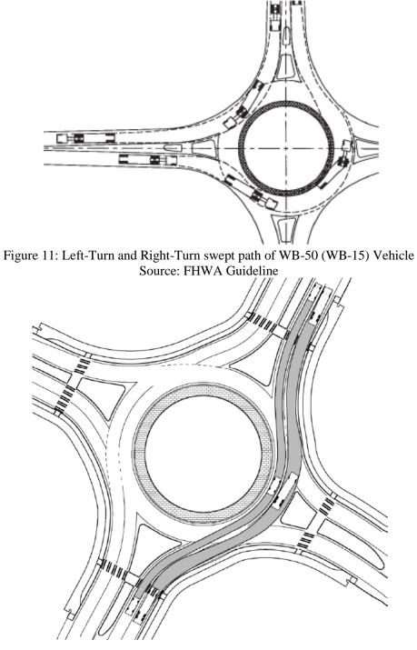
Figure 12: Bus and Passenger Car Swept Paths, Multilane Roundabout Source: NCHRP Report 672
