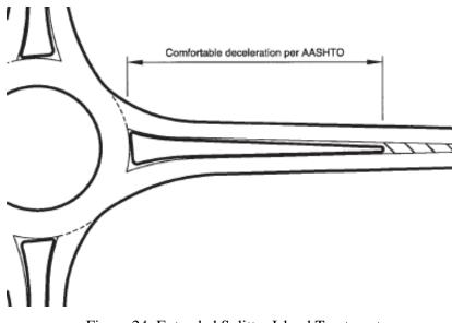
Figure 24: Extended Splitter Island Treatment Source: NCHRP Report 672
