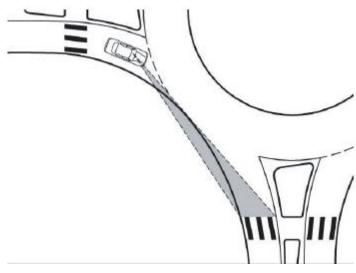
Figure 23: Stopping Sight Distance to Crosswalk on Exit Source: NCHRP Report 672
