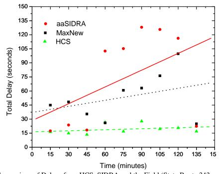
Figure 33: Comparison of Delays from HCS, SIDRA and the Field (State Route 343 and E Main St) Figure 34 and Figure 35 show the delay values from the HCS and SIDRA plotted against field values. From the graphs, it can be seen that the results obtained from SIDRA appeared a better fit with the field data compared to HCS. It can be concluded that SIDRA is more suited for the prediction of delays at Nevada roundabouts.
