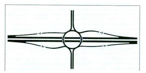
Figure 6: Diamond Interchange with Roundabout at Single Ramp Terminal Intersection
