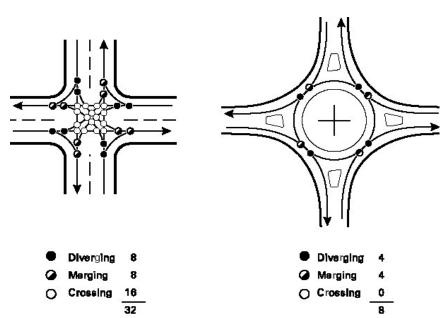
Figure 3: Comparison of Vehicle-Vehicle Conflict Points for Four-Legged Intersection and Roundabout Source: NCHRP Report 672
