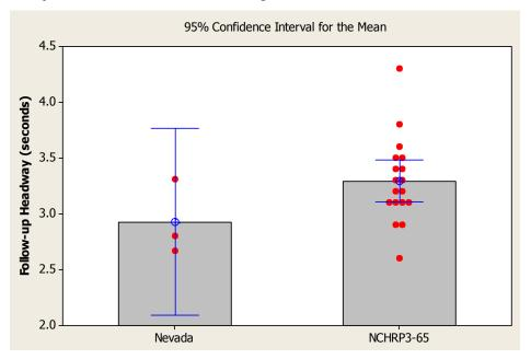
Figure 30: Comparison of Follow-up Headways from Nevada and NCHRP 3-65 (Single-Lane Sites) 95% Confidence Interval for the Mean
