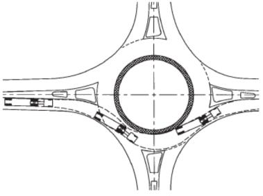
Figure 10: Through-Movement Swept Path of WB-50 (WB-15) Vehicle Source: FHWA Guideline
