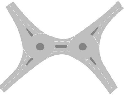
Figure 2: Illustration of a Double Roundabout with Short Central Link
