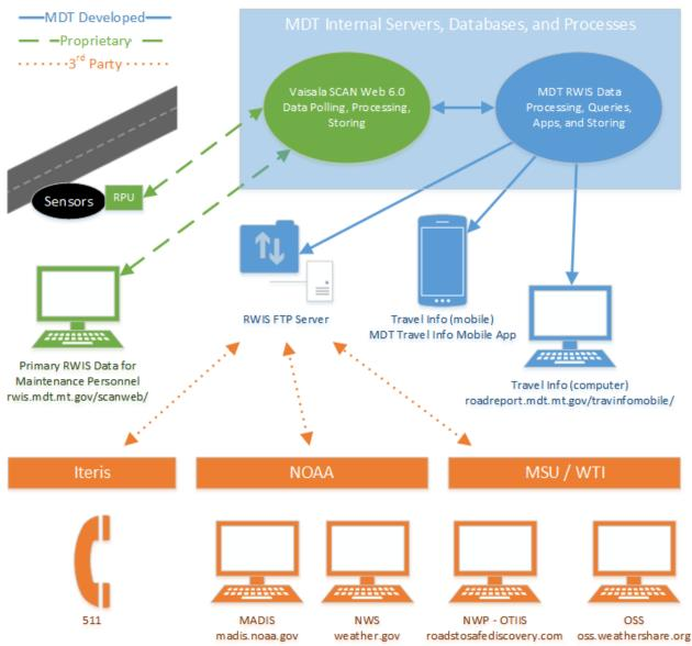
Figure 35: System Architecture
