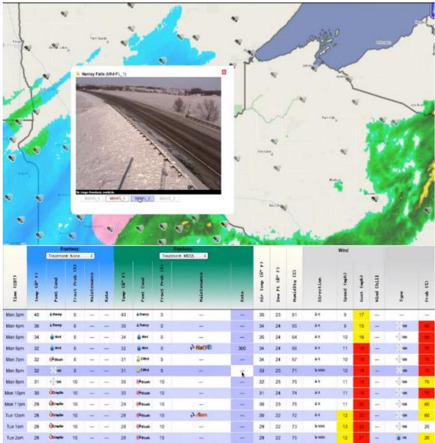
of the functionality of the ClearPath Weather software with a map and camera view (top) and a table of forecast weather and pavement conditions and MDSS actions (bottom).
