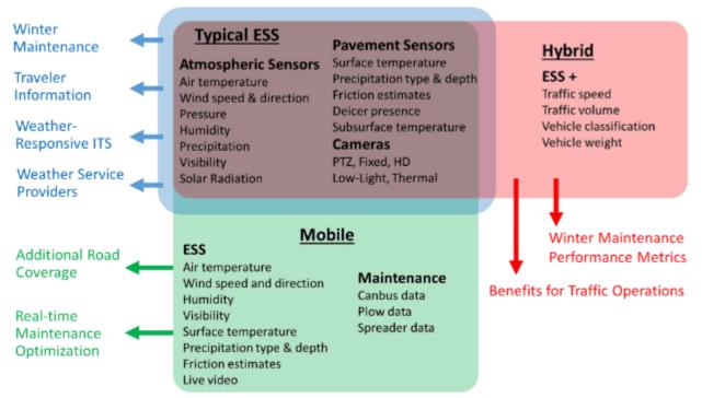
Figure 1: RWIS Components and Uses
