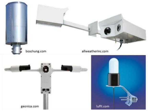
Figure 6: Precipitation Sensors
