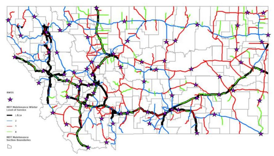
\*map does not show 7 satellite maintenance sections that operate within certain of the 118 sections (125 sections total) Figure 54: Maintenance Sections, RWIS sites, and Winter Maintenance Service Levels
