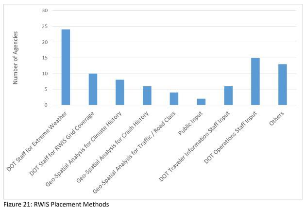
Figure 21: RWIS Placement Methods
