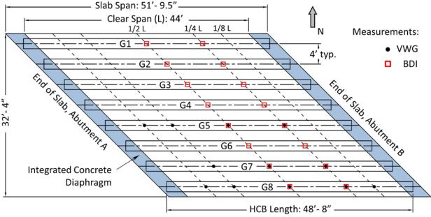
Figure 7. Bridge Nomenclature With Instrumentation Overview (Plan View)
