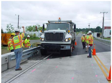
Figure 20. Static Load Testing with Truck Guided Along Wheel Path A
