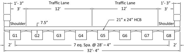
Figure 6. Tides Mill Stream – HCB Bridge Cross-Section
