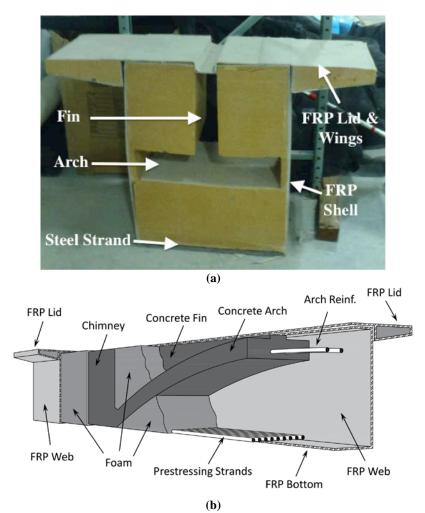
Figure 2. Hybrid Composite Beam (a) Cross-Section and (b) Isometric System
