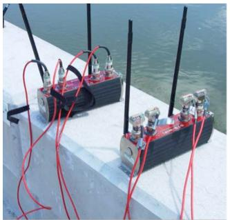
Figure 16. Wireless BDI Node with Intelliducer Plugs
