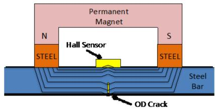
Figure 40. Magnetic Flux Leakage Theory. Adapted from Civitillo (2014).
