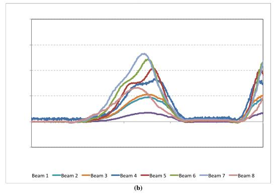
Figure 21. Time Series Strain Data (All Beams) – Static Loading (a) Load Case A1 and (b) Load Case F1
