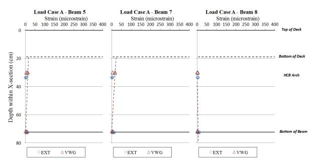
Figure 35. Quarter-span Strain Profiles Load Case A
