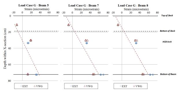
Figure 33. Mid-span Strain Profiles Load Case G
