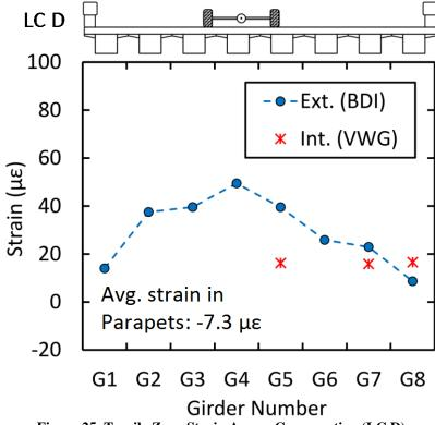
Figure 25. Tensile Zone Strain Across Cross-section (LC D)
