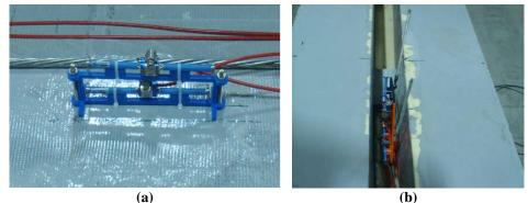
Figure 10, Stacked Strain Gauge Configuration: (a) Concrete Arch VWG Frame at Mid-span and (b) Additional Rosette Configuration at Eighth-span
