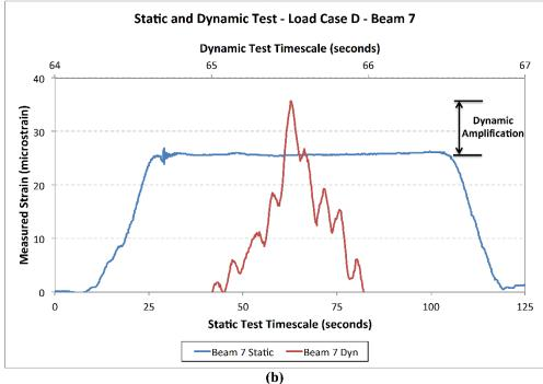
Figure 39. Maximum Dynamic Amplification Response (a) Load Case B and (b) Load Case D
