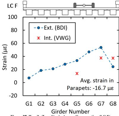
Figure 27. Tensile Zone Strain Across Cross-section (LC F)
