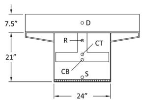
Figure 8. General Vibrating Wire Gauge Locations Through the Depth
