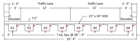
Figure 12. Tides Mill Stream Bridge Cross-Section With Midspan External Strain Gauge Configuration
