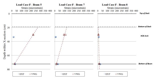
Figure 36. Quarter-span Strain Profiles Load Case F
