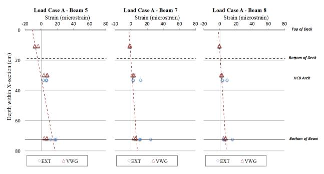
Figure 31. Mid-span Strain Profiles Load Case A
