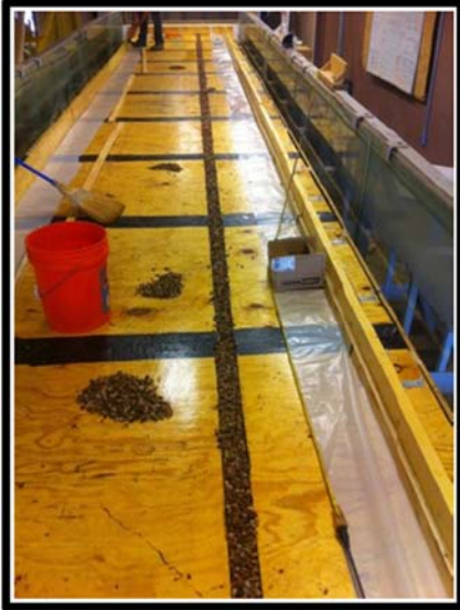
a) Underdrain Slot Backfilled with Aggregate
