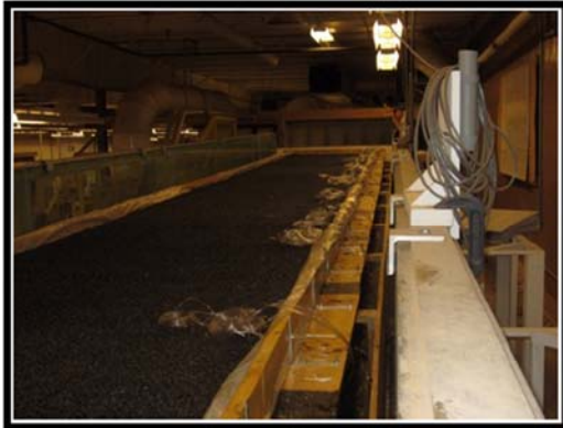
c) Manometer Tubes Feeding to Manometer Board
