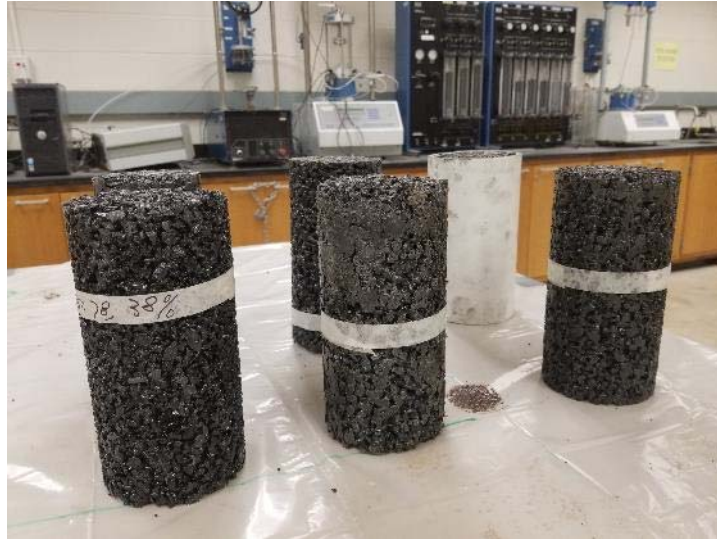
Figure 47. Specimen used in the hydraulic conductivity test
