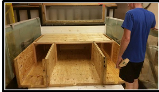
b) Placement of Interior Flume Channel Upstream Row
