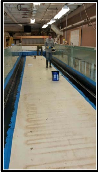
a) Water Sealing Edges of Outer Flume Channel-With Painter's Tape
