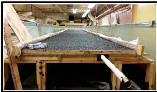
b) PFC Layer With Underdrain Shown
