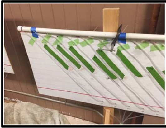
a) Manometer Board
