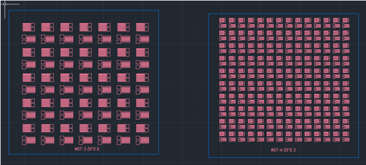
Figure 67. Photomask of temperature sensor
