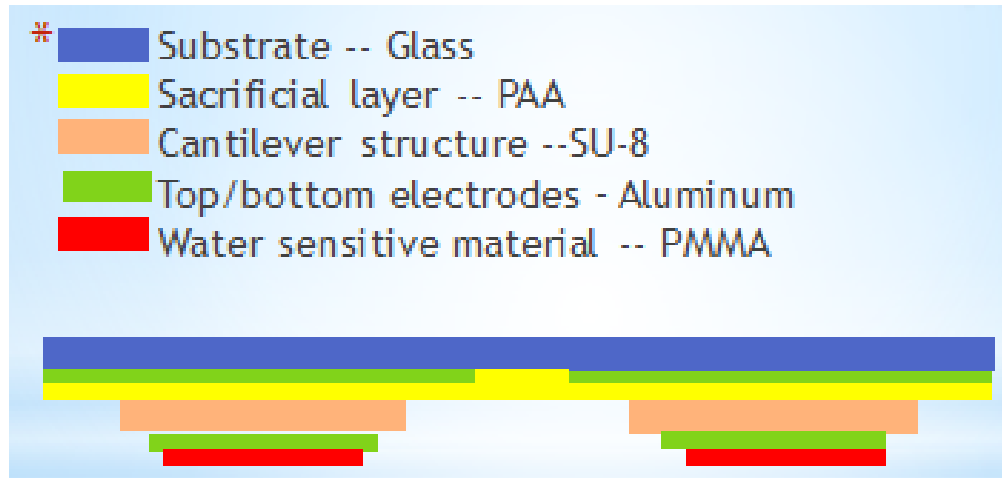
Figure 1. Concept design of Generation 1 MEMS moisture sensor
